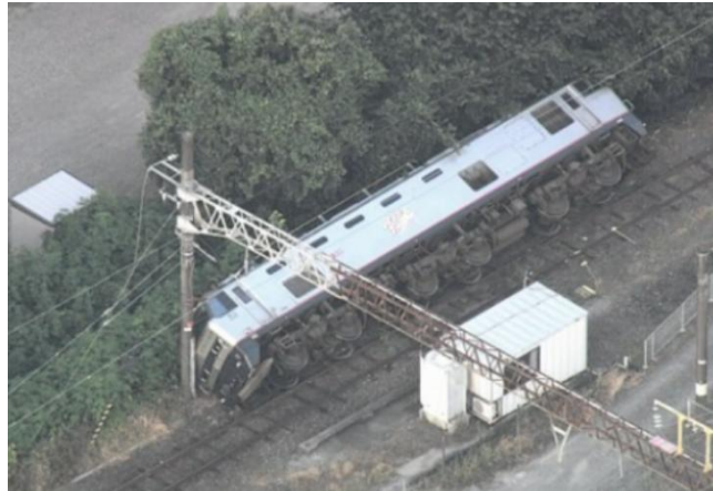
Figure 56. Locomotive and freight car derailment ( Link 105 )
