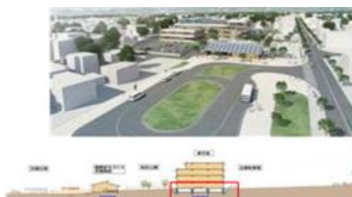
(b) Seismic design: Base-isolated foundation [link 83 ]
