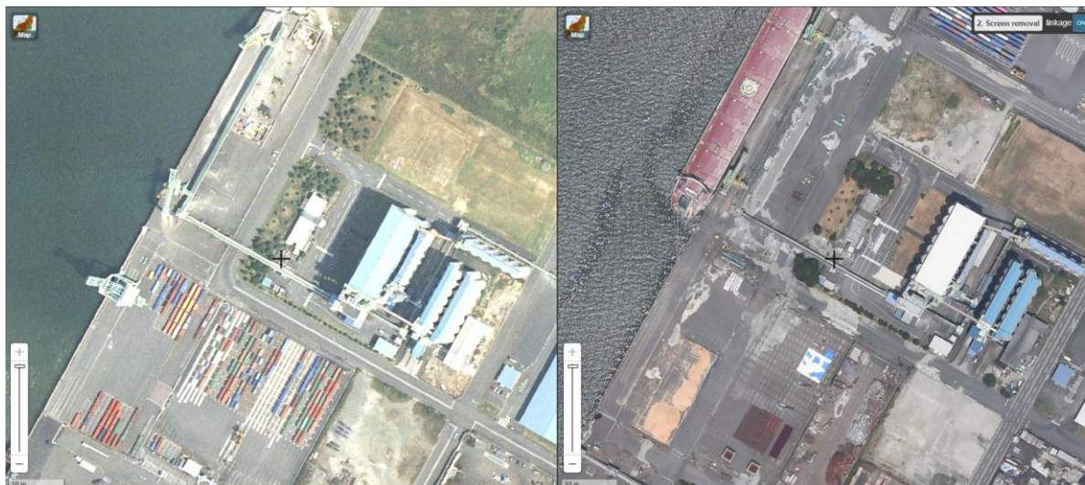
Figure 25. Comparison of satellite imagery of Yatsushiro Port before and after the 2016 Kumamoto Earthquake sequence, illustrating earthquake-induced ground deformation and liquefaction on reclaimed port areas. (Source: Geospatial Information Authority of Japan (GSI) online map service 37 )
