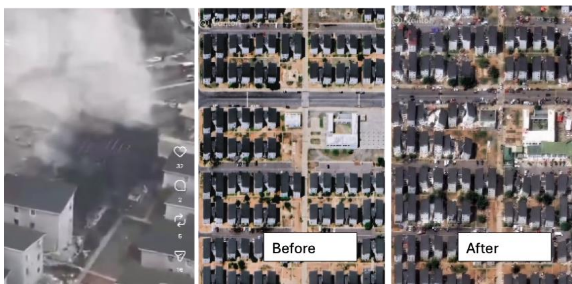
Figure 23. Damage to a development in Playa Grande built during the Great Mission Housing Programme 2011-13. Building on fire (left, Social Media ) and many collapses (middle to right, source: Vantor Satellite Imagery). These structures are steel frame and steel stud, rather than the predominant concrete elsewhere in the region.
