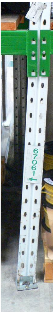
Figure 4 Down-aisle distortion of post
