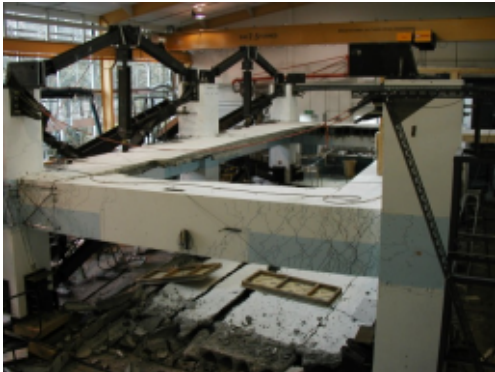
(c) The frame after the floor collapsed
