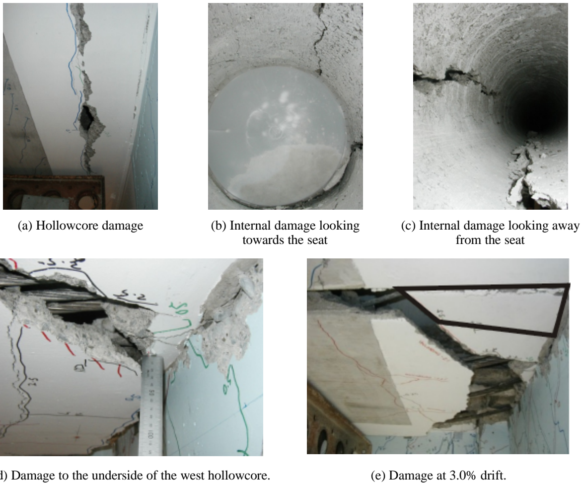
Figure 4. Observed damage during Phase II testing
