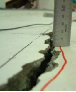
(c) Vertical offset after the tear formed (-2.0% drift)
