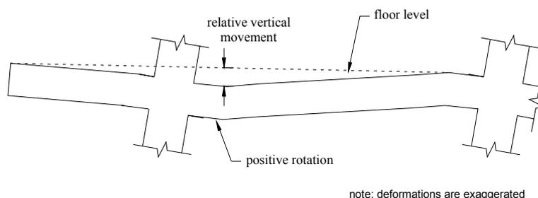
Figure 8: Illustration of vertical movement between floor and beam.
