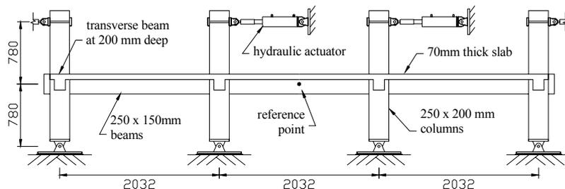
Fig. 2: Test arrangement of 3-bay frame with composite slab (Fenwick *et. al.* 1995).
