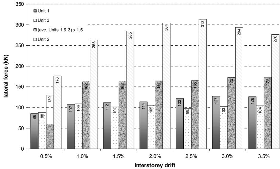
Fig. 5: Lateral strength comparison of test units.
