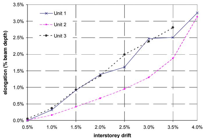
Fig. 6: Elongation of beams.
