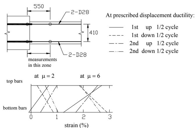
Fig. 1: Elongation of reinforcement in plastic hinge zone (Fenwick & Megget 1993).
