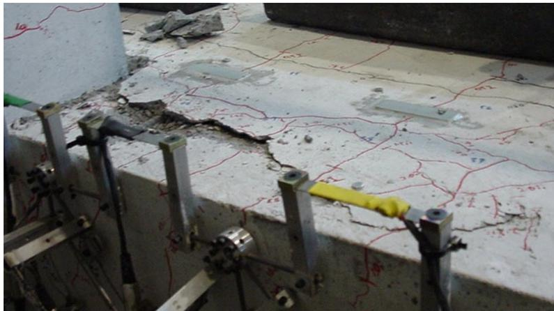
Figure 7: Relative vertical movement of slab and beam.
