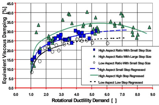
Figure 3 Beam Flexural Damping
