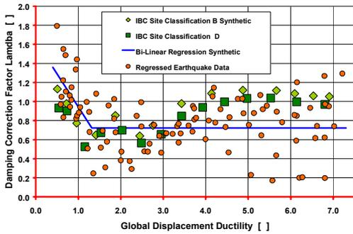
Figure 7 Correction Factor "Lambda" Data Regression
