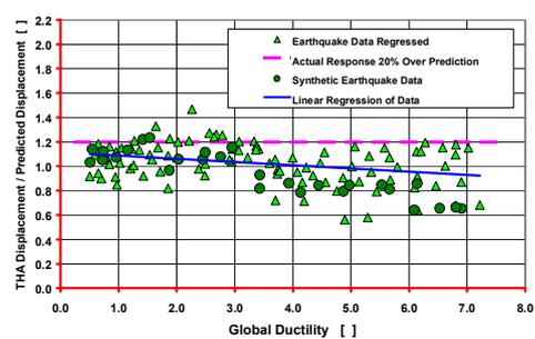
Figure 10 Calibrated Substitute Structure Prediction Accuracy
