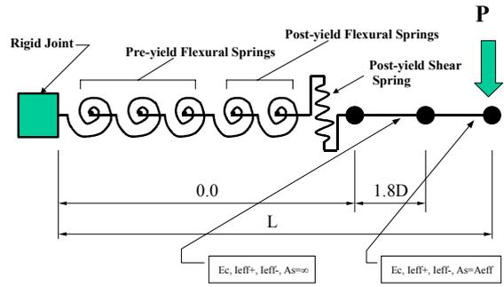
Figure 4 Beam Hinge Composite
