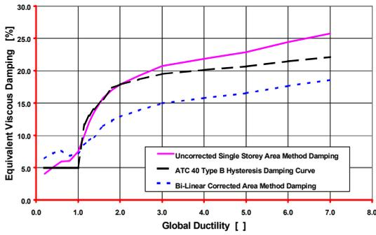
Figure 5 Single Storey Structure Global Damping Curves.
