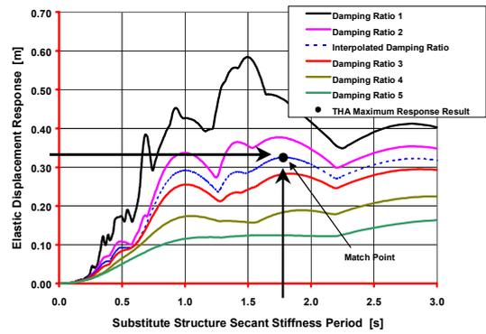
Figure 6 Calibration Method
