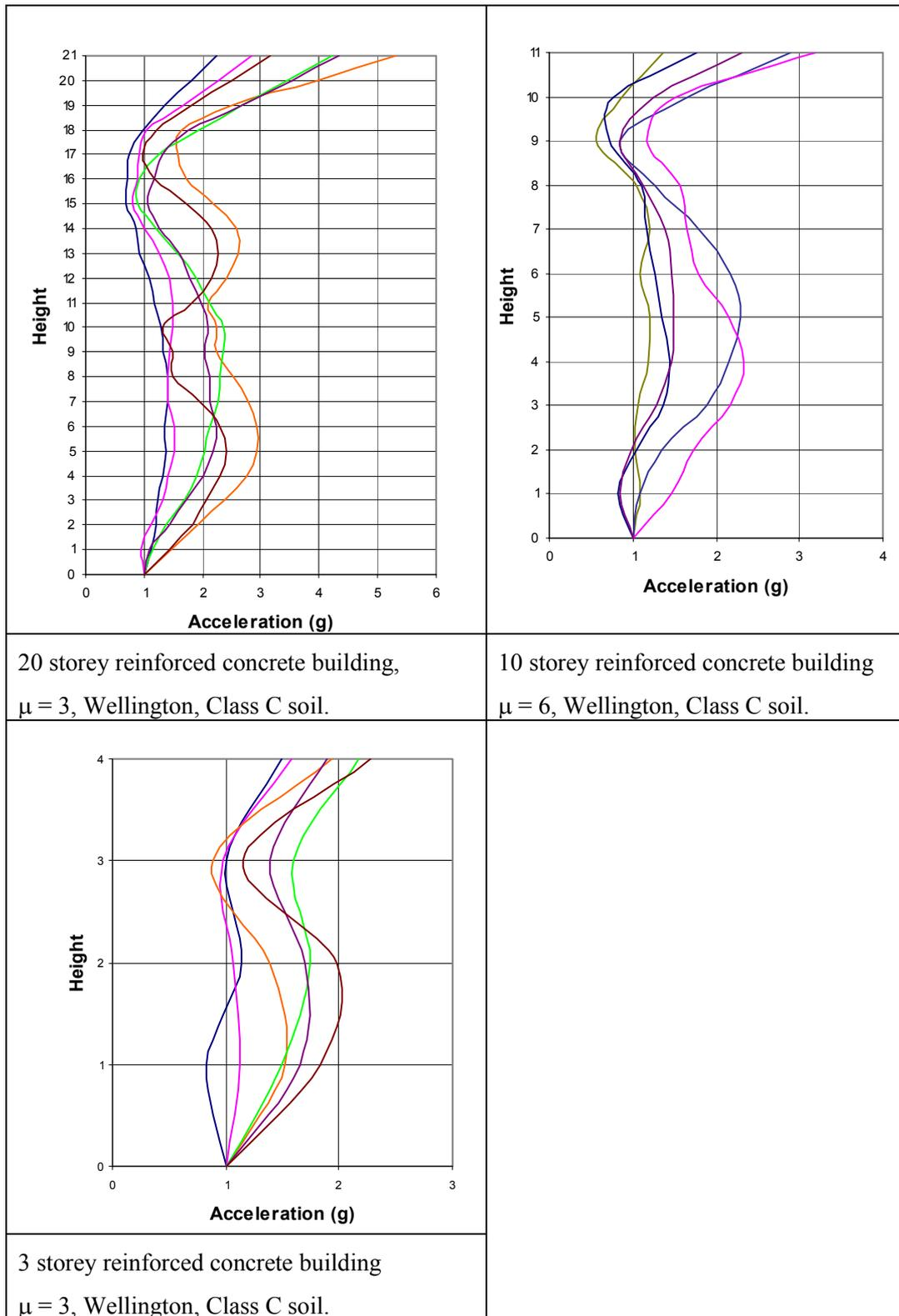
Figure 3. Floor accelerations for example buildings.
