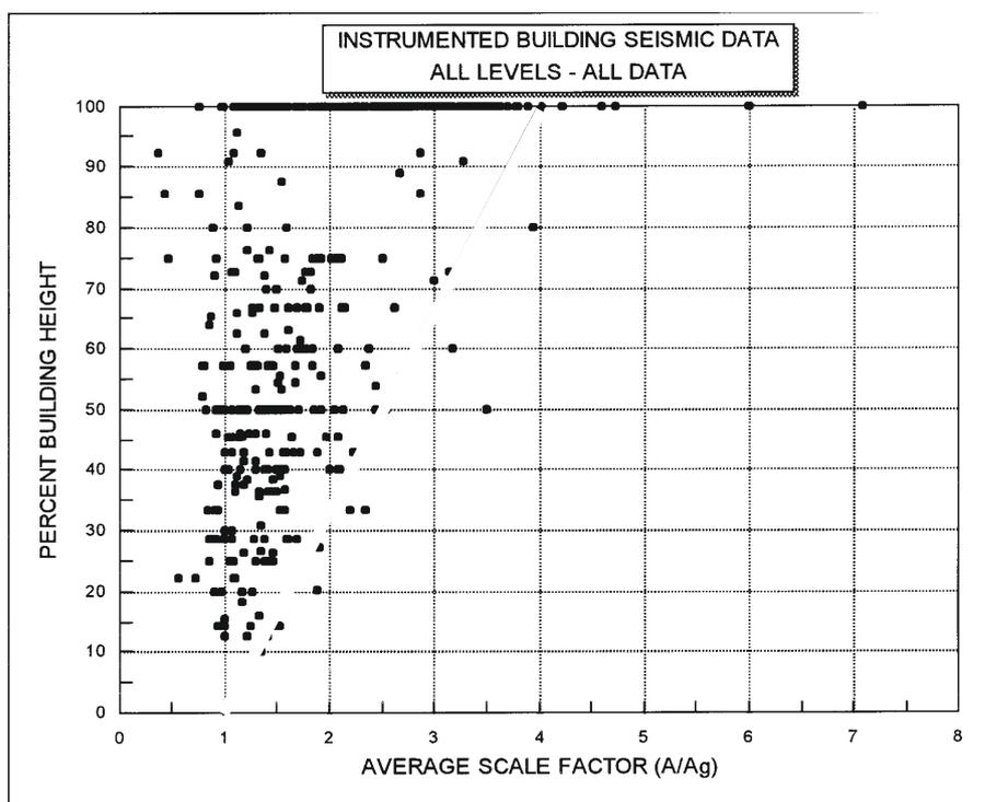
Figure 4. Recorded floor accelerations. From Drake and Bachman (1995)
