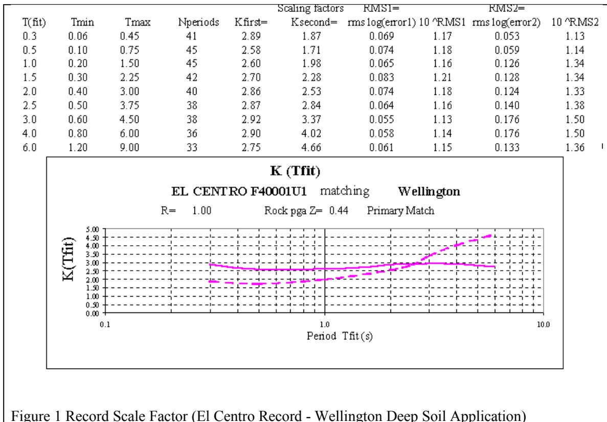
Figure 1 Record Scale Factor (El Centro Record - Wellington Deep Soil Application)
