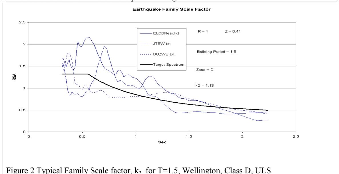
Figure 2 Typical Family Scale factor,  $k_2$  for  $T=1.5$ , Wellington, Class D, ULS
