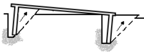
Figure 10. Observed failure mechanism.
