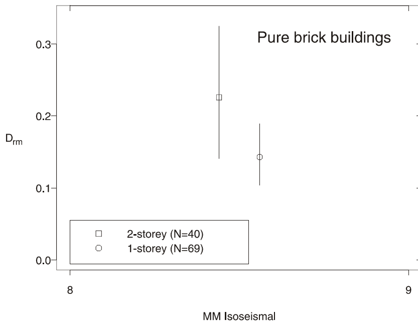
Figure 3. D_{rm} and its 95% confidence limits for one and two-storey non-domestic pure brick buildings in the MM8 intensity zone of the June 1942 Wairarapa earthquake.
