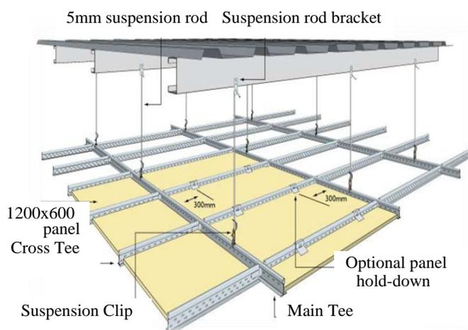
(b) Suspended system: Two-way exposed
