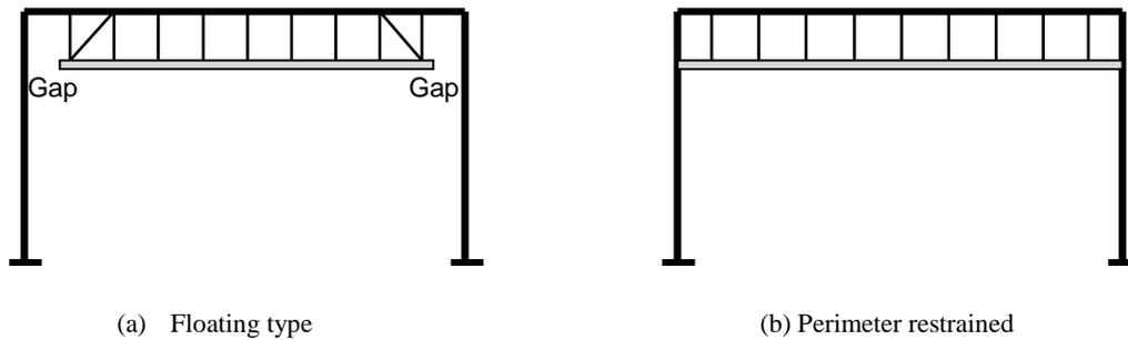
Figure 2: Common installation methods for suspended ceilings.
