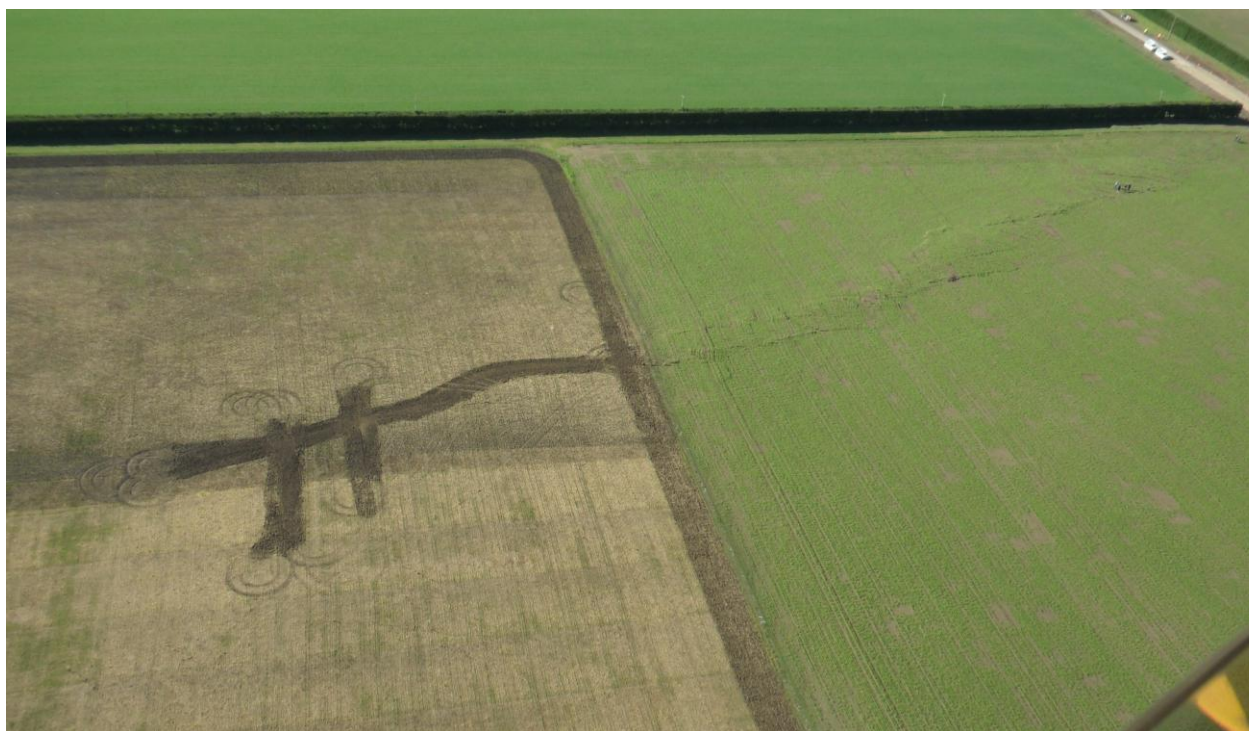
Figure 2 : Early cultivation of the Greendale fault. Several passes with roto-crumbler cultivation has been used in the left paddock; whilst the paddock on the right shows the unaltered surface rupture.
