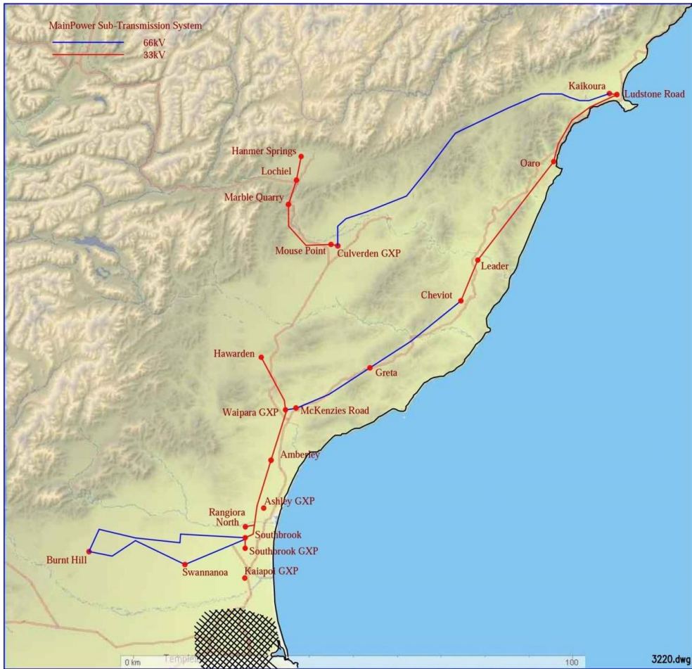
Figure 3: MainPower Subtransmission Network.
