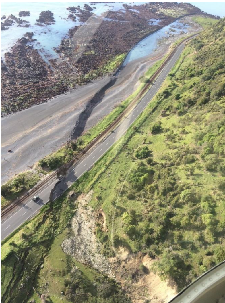
Figure 12: Aerial view of a southwestern strand of the Papatea Fault surface rupture across State Highway 1 and the SIMT line. This scene lies about 100 m south of that shown in Figure 10 and 900 m southwest of the Figure 11 view of the northeastern strand of the fault (view to the south; photograph from Chris Hayles).
