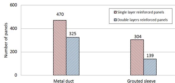
Figure 21: Quantity of each type of reviewed grouted wall-to-foundation connection in single layer and double layer reinforced walls.
