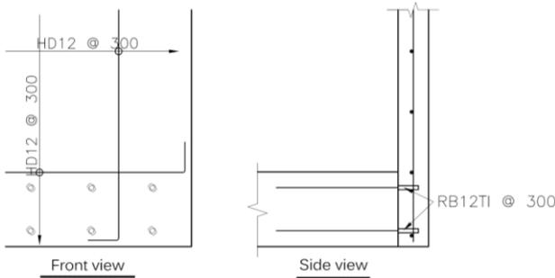
\* foundation reinforcement is not shown
