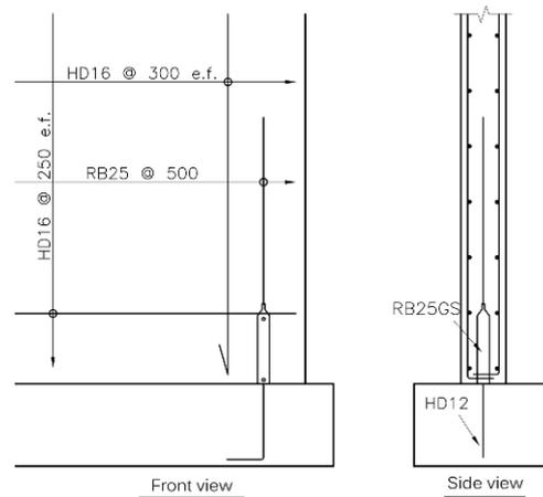
Figure 16: An example of a double layer reinforced panel with a grouted sleeve connection.
