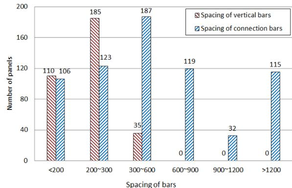
Figure 12: Spacing of panel vertical bars and connection bars (mm).
