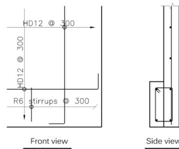
\*foundation reinforcement is not shown
