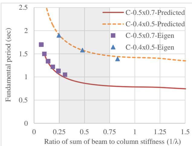
(c) 8 Storey frame with 4 bays and 6m span
