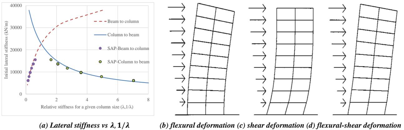
Figure 4: Lateral stiffness vs beam-column, column-beam relative stiffness and lateral deformation of frame buildings [22].
