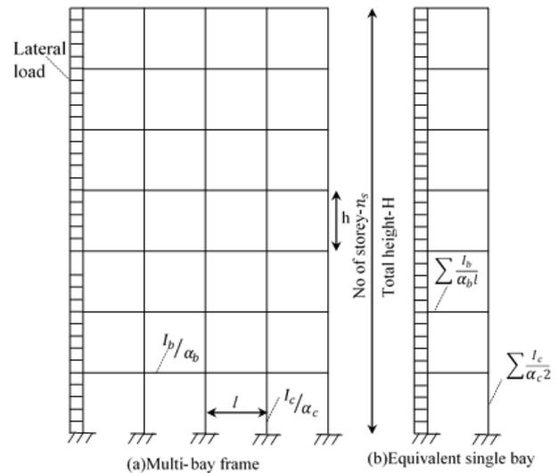
Figure 2: Condensation of a multi bay frame into an equivalent single bay frame.
