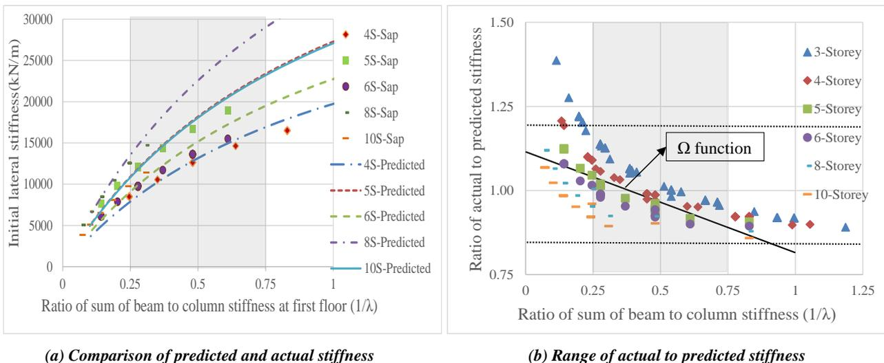
Figure 5: Comparison of predicted and actual lateral stiffness with  $\gamma=1$ .
