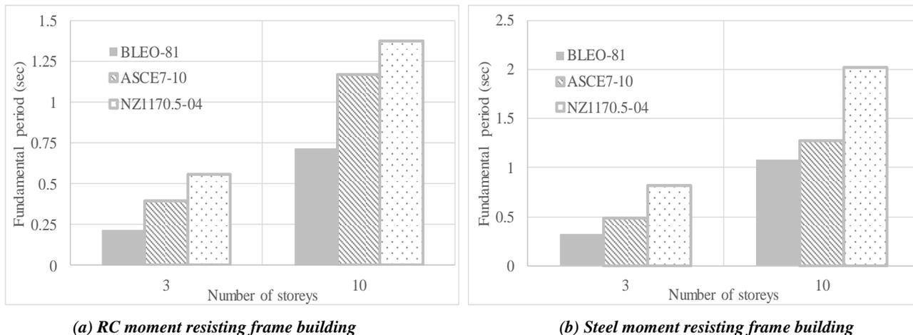
**Figure 1: Fundamental period calculated using empirical equations in different standards.**
