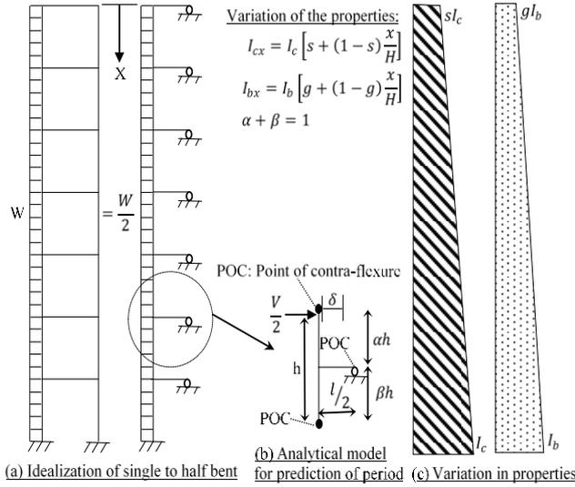
**Figure 3: Modified Macleod's model to predict the fundamental period of a frame building.**
