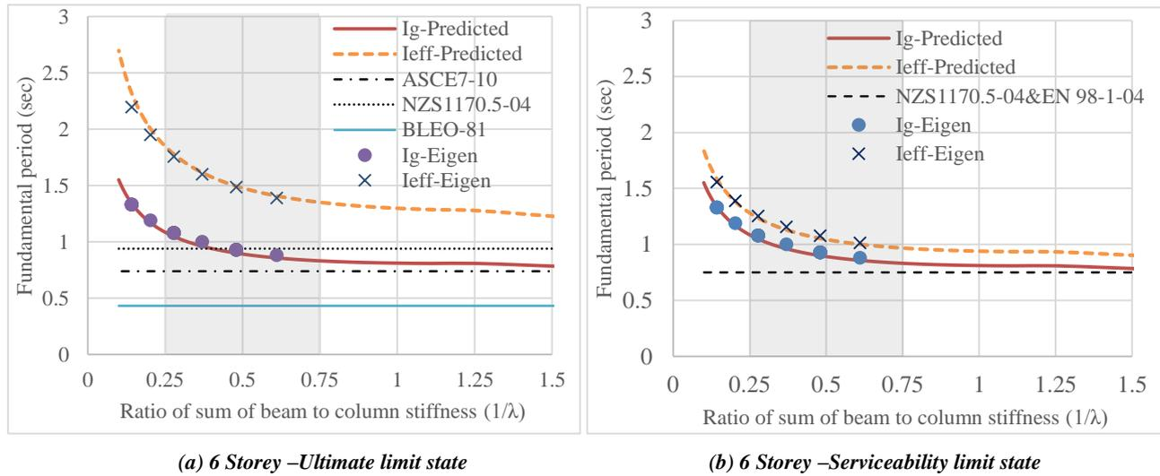
Figure 15: Limitations of empirical equations in prediction of period (i.e. effective properties).
