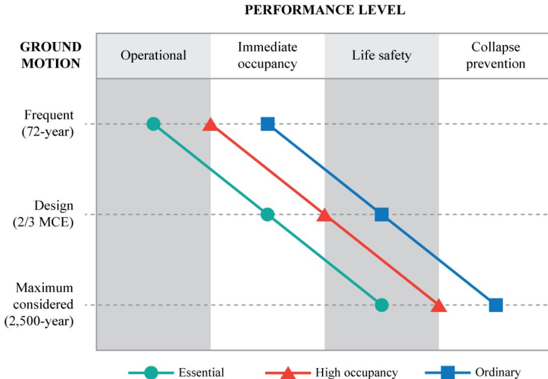
*Figure 1: Seismic performance objectives for different building occupancies specified in the NEHRP Recommended Provisions (adapted from BSSC 2003 [11] and BSSC 2009 [9]).*
