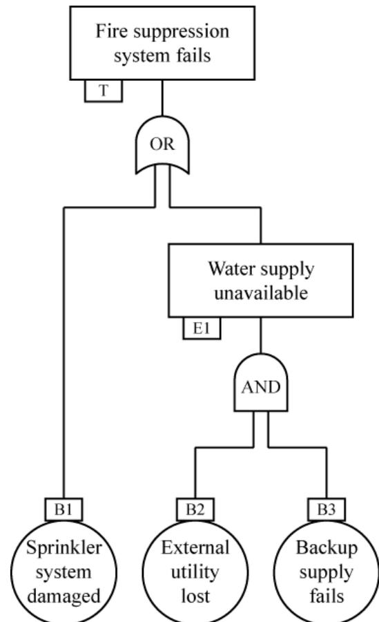
**Figure 2: Example of a simple fault tree that captures failure of a hypothetical fire suppression system in a building.**
