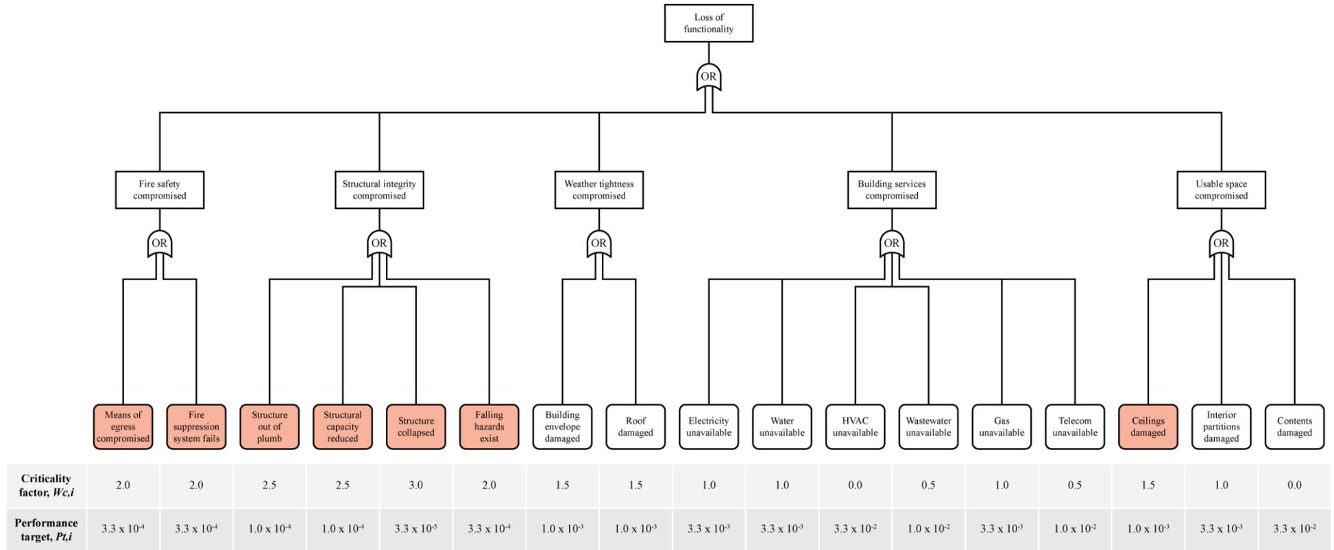
Figure 5: Fault tree for capturing loss of functionality in a generic commercial building, including criticality factors ( $W_{c,i}$ ) and performance targets ( $P_{t,i}$ ) for each “basic” event corresponding to a global resilience objective ( $P_{t,sys}$ ) of 10% probability of losing functionality in ground shaking with a particular return period.
