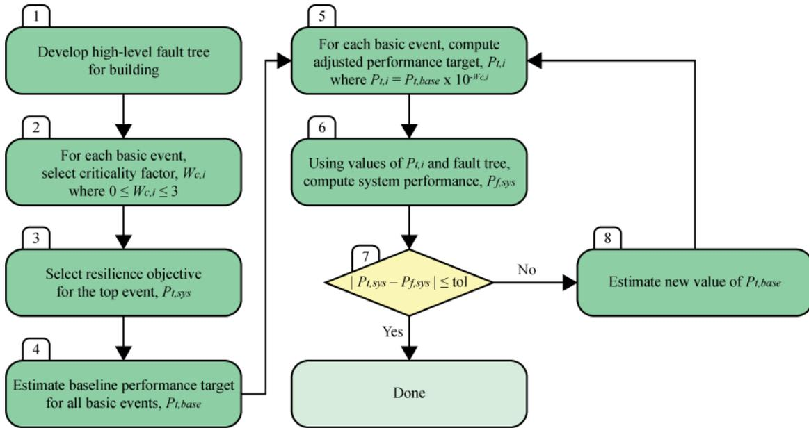
**Figure 3: Methodology for computing risk-consistent performance targets for basic events from a global resilience objective for the top event in a fault tree.**
