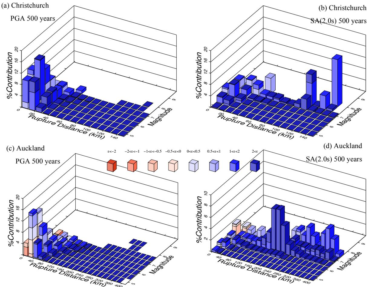
**Figure 5: Seismic hazard deaggregation illustrating the dominant seismic sources contributing to the total seismic hazard: (a) Christchurch – PGA; (b) Christchurch SA(2.0s); (c) Auckland – PGA; and (d) Auckland SA(2.0s). It can be seen that small magnitude close proximity sources dominate the PGA hazard, while faults with greater magnitudes and high rates at large distances dominate the SA(2.0s) hazard.**
