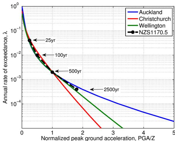
**Figure 3: Normalization of the site-specific hazard results in Figure 1 by the 500 yr return period in order to illustrate the various shapes of the hazard curves in comparison with the return period factor,  $R$ , in NZS1170.5.**
