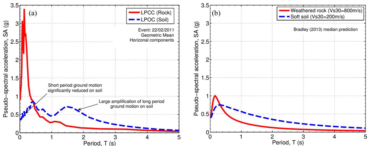
**Figure 4: Illustration of the consideration of nonlinear site effects in empirical GMPEs: (a) observed horizontal response spectra at rock and soil sites in Lyttelton Port in the 22 February 2011 Christchurch earthquake [14]; and (b) nonlinear site effects based on the Bradley (2013) GMPE median prediction.**
