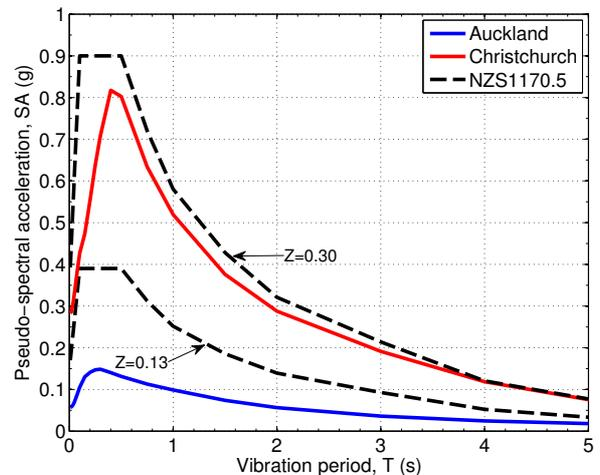
Figure 2: Site-specific UHS for the 500 year return period at generic site class D sites in Auckland and Christchurch in comparison with the NZS1170.5 design Z values (using Z = 0.13 and 0.30, respectively).
