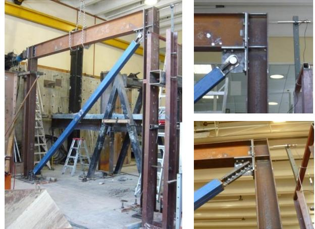
Figure 11: Sub-assembly test model at the laboratory.
