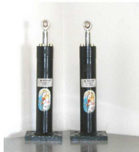
Figure 10: Prototype ring spring devices used in the experimental testing.
