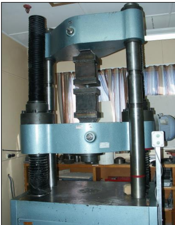
Figure 7: Specimen arrangement in Shimadzu UTM for testing bar heads on bars recovered from Kaiapoi Railway River Bridge.
