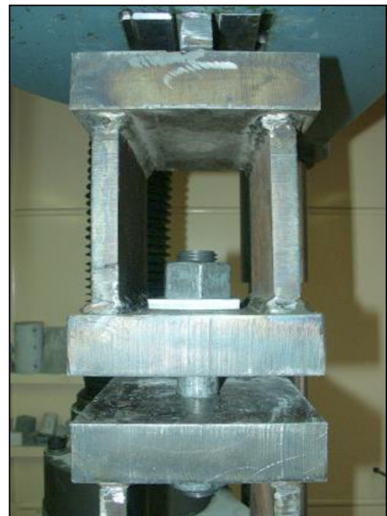
Figure 8: Bar head test set-up in Shimadzu UTM.
