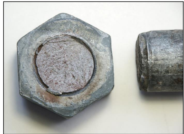
Figure 10: Failure in bar head test.
