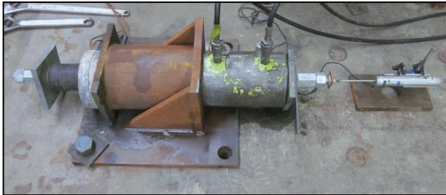
Figure 6: Hydraulic jack loading system set-up for Reidbar RB25 tests. Deflection measurement gauge is at the right end of the bar. Gauge was repositioned to be alongside the jack prior to bar failure.
