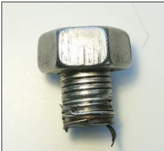
Figure 12: Failure of A4-70 (LE) nut in RS38 assembly test. Note the distortion across the width of the nut.
