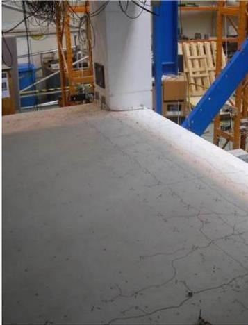
(c) Timber infill cracks, less than 0.45 mm.
