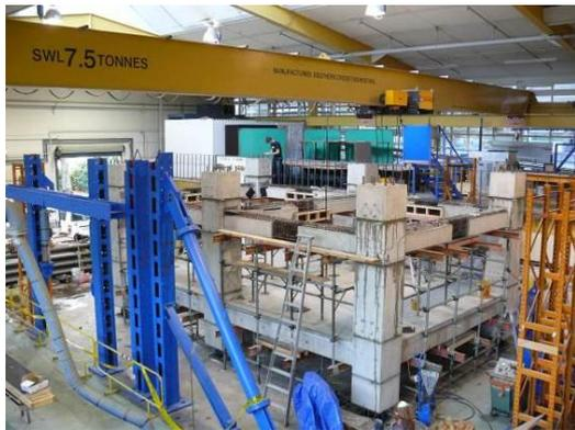
(c) Second floor precast components being grouted.
