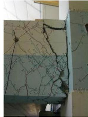
(b) Monolithic reinforced concrete plastic hinge damage (MacPherson, 2005).
