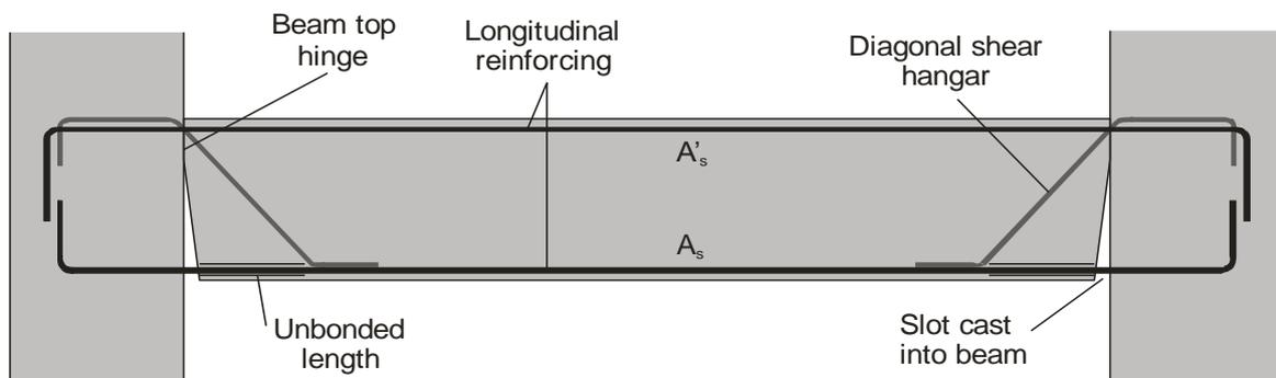
*Figure 1: Diagram of a slotted reinforced concrete beam.*
