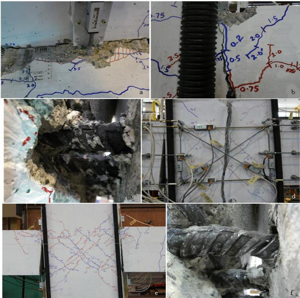
**Figure 6:** *Damage during 4.5% and 5.5% drift cycles (a) Crack above west hinge; (b) Full length crack through west hinge; (c) Cone pull out bottom west of joint; (d) Steeply inclined joint shear cracks; (e) Joint cracking and strain penetration; (f) Bar fracture.*
