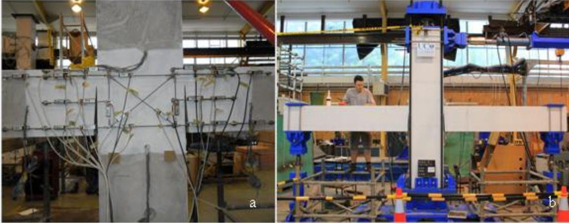
Figure 3: (a) Linear potentiometer layout; (b) Specimen in testing rig.
