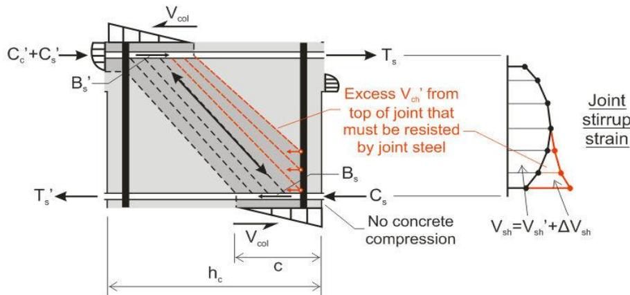
Figure 2: Interior slotted beam joint mechanism proposed by Au (2010).
