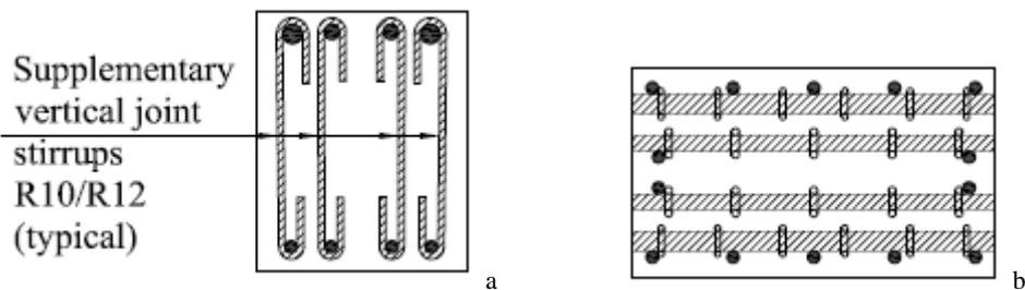
Figure 4: Supplementary vertical joint stirrups layout. (a) Beam section; (b) Column section.
