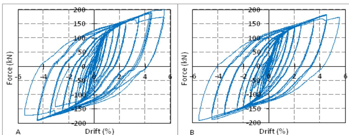
Figure 5: Lateral force vs. Inter-storey drift for Specimen A and B.
