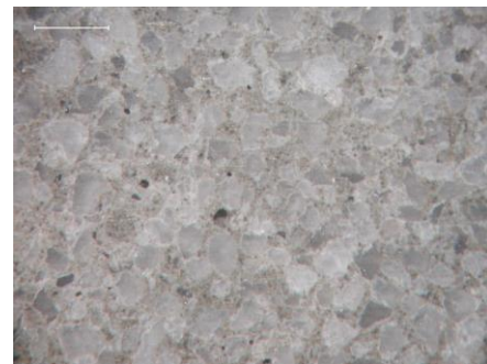
Figure 10: View of the surface of synthetic sandstone through an optical electron microscope.
