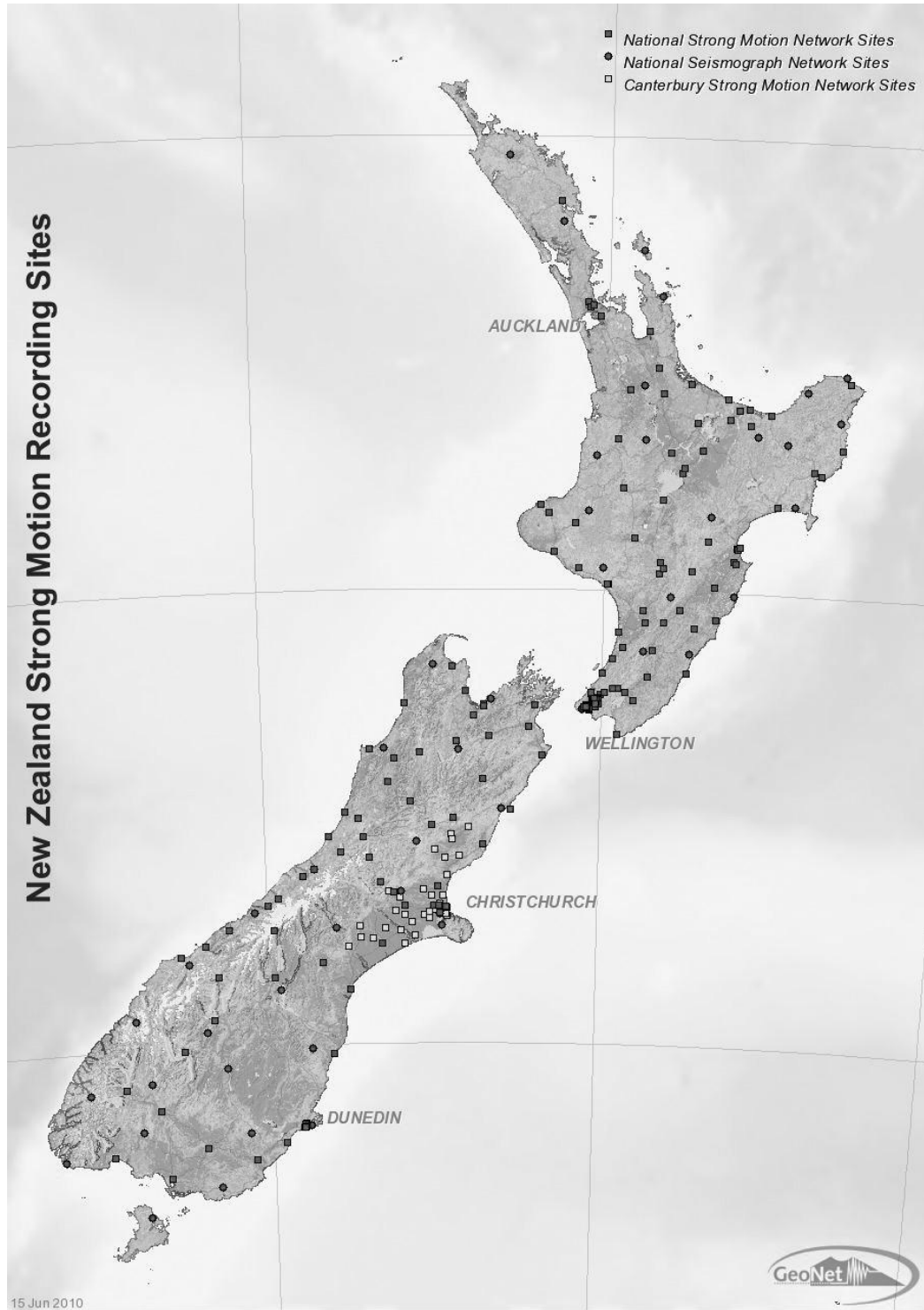
Figure 1: New Zealand strong-motion recording sites: National Strong-Motion Network sites(solid squares); National Seismograph Network sites(circles); and Canterbury Network sites(light squares) as in Figure 2.
