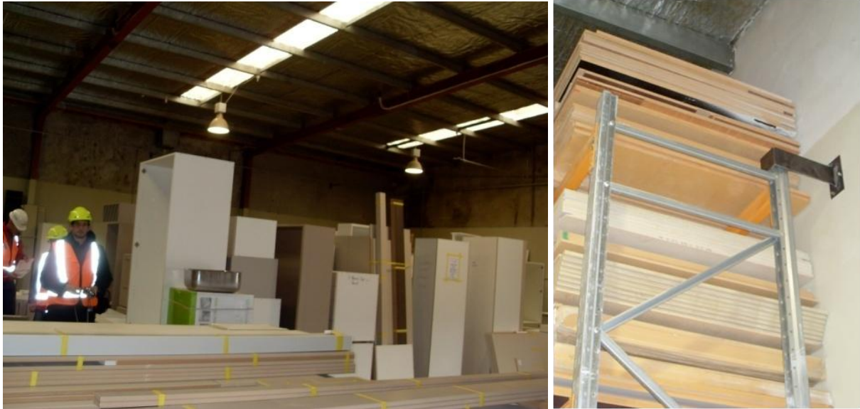
Figure 2: Undamaged stock and storage rack bolted to wall in Kitchen cabinet manufacture site. Source: D. Mukai.
