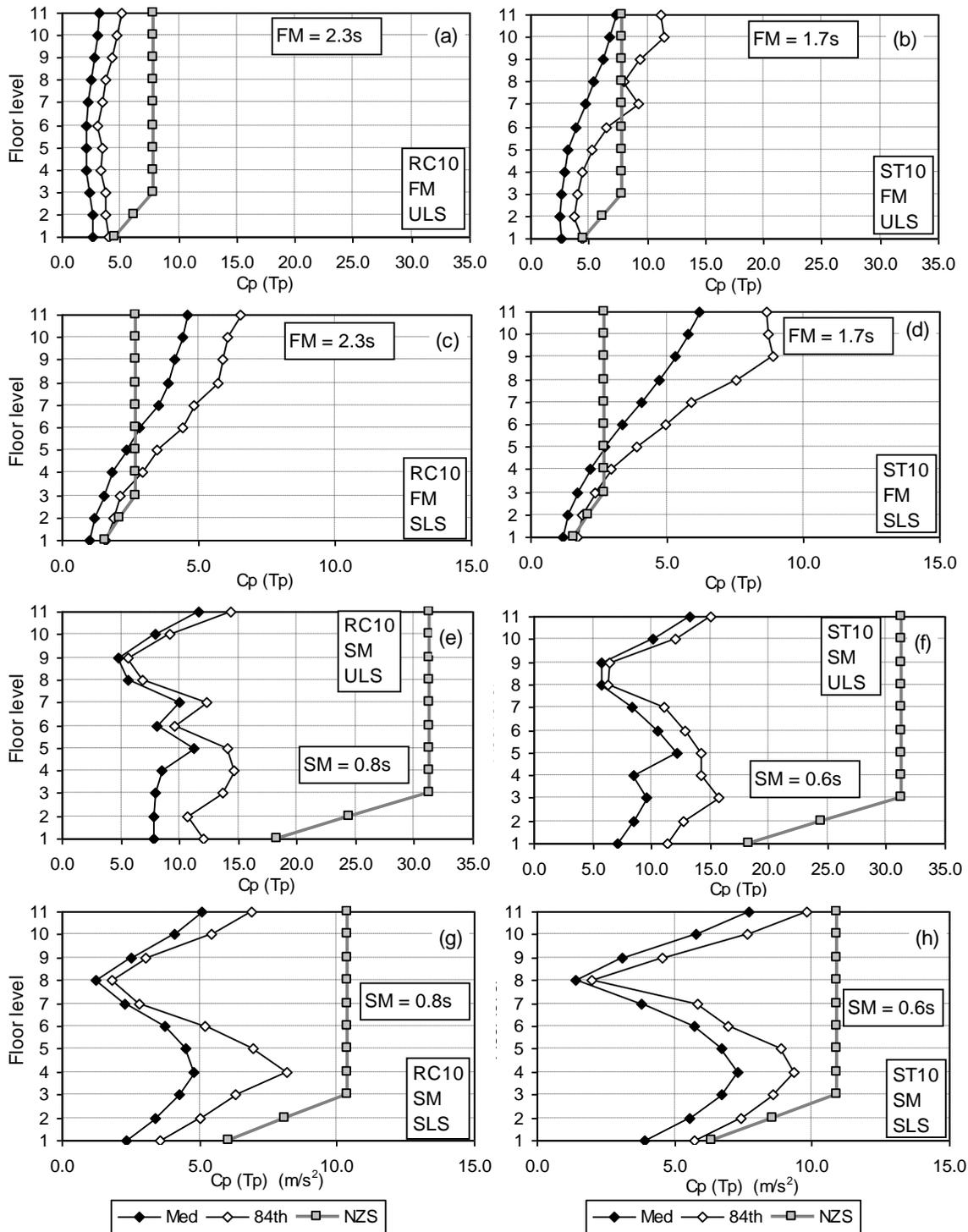
Figure 10: Acceleration demands ( $m/s^2$ ) on components in high-rise buildings under ULS and SLS intensities.
