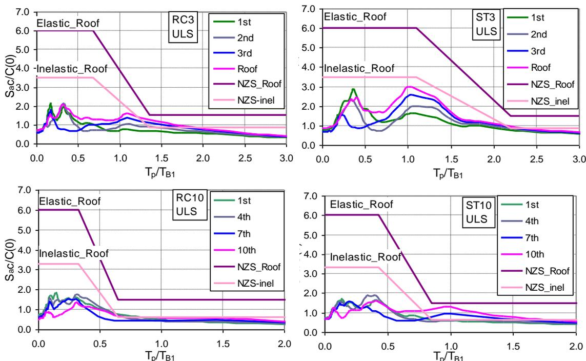
Figure 8: Less spectral amplification near fundamental period range for ULS intensities.
