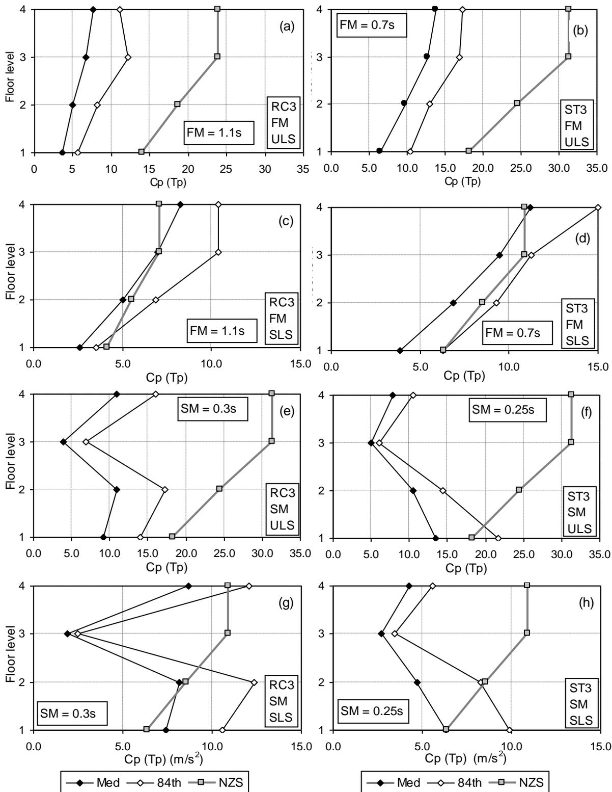
Figure 9: Acceleration demands ( $m/s^2$ ) on components in low-rise buildings under ULS and SLS intensities.
