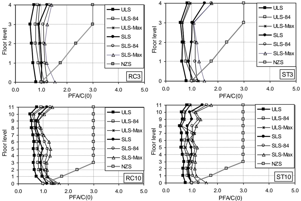
**Figure 4: Floor height coefficient distributions for ULS and SLS intensities.**
