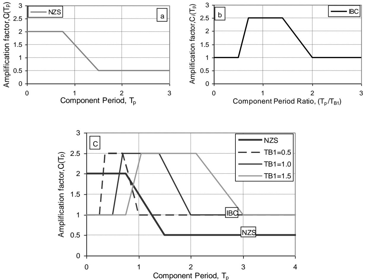
**Figure 2: Component amplification factor: (a) NZS provisions independent of  $T_{B1}$ ; (b) IBC provisions; (c) comparison of NZS provisions with IBC provisions for  $T_{B1} = 0.5s, 1.0s, \text{ and } 1.5s$ .**
