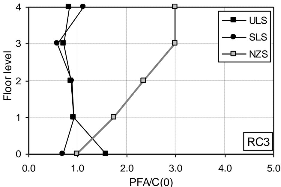
*Figure 12: Floor height coefficient distributions under slab events.*
