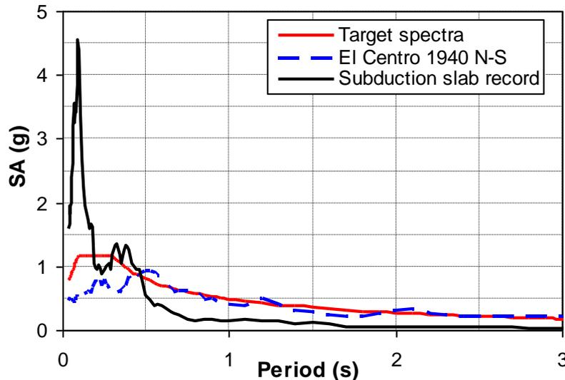
**Figure 11: A clear illustration of record scaling and the different frequency contents between a shallow crustal record (El Centro 1940) and a subduction intra-slab record.**
