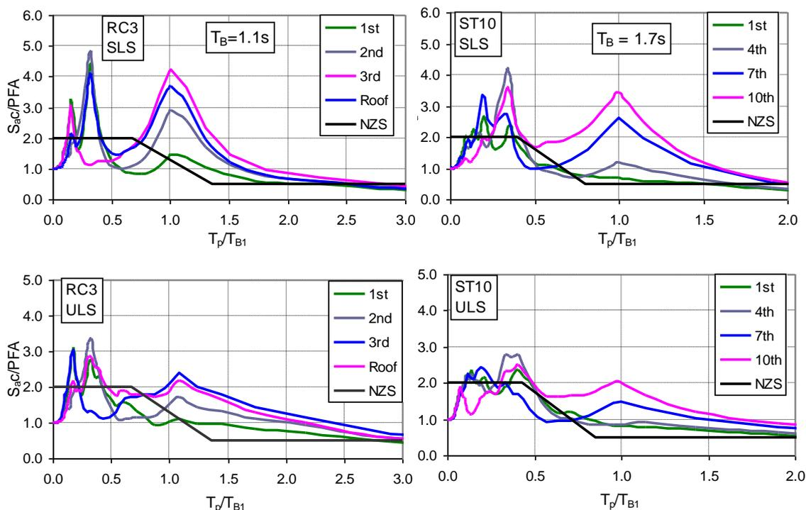
Figure 5: Component amplification factor for low and high-rise buildings under SLS and ULS conditions – the analytical CAF exceeds the NZS recommended envelope.
