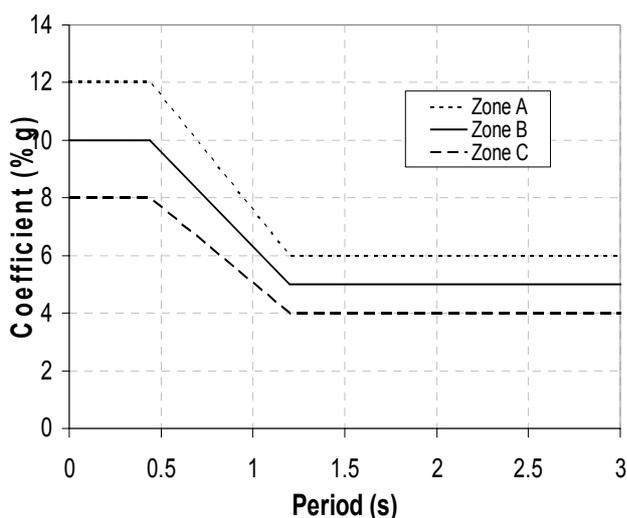
Figure 1. NZSS 1900: basic lateral force coefficients.
