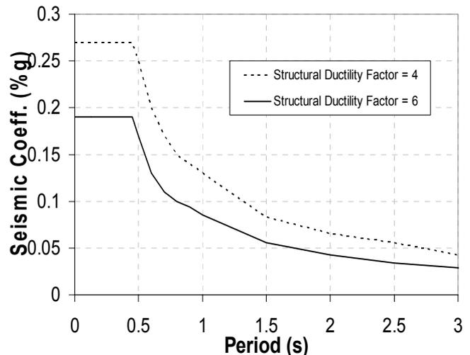
Figure 3. NZS 4203:1992, Acceleration coefficient for soil class B
