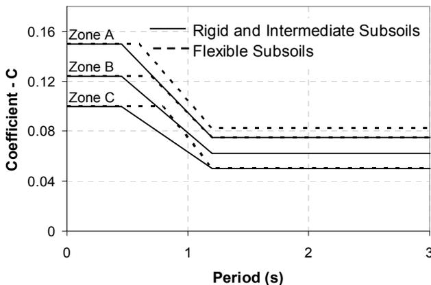
Figure 2. NZS 4203:1976 and 1984, basic seismic coefficient
