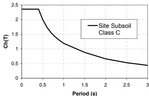
Figure 4. Spectrum shape factor for NZS1170.5 with class C soils.
