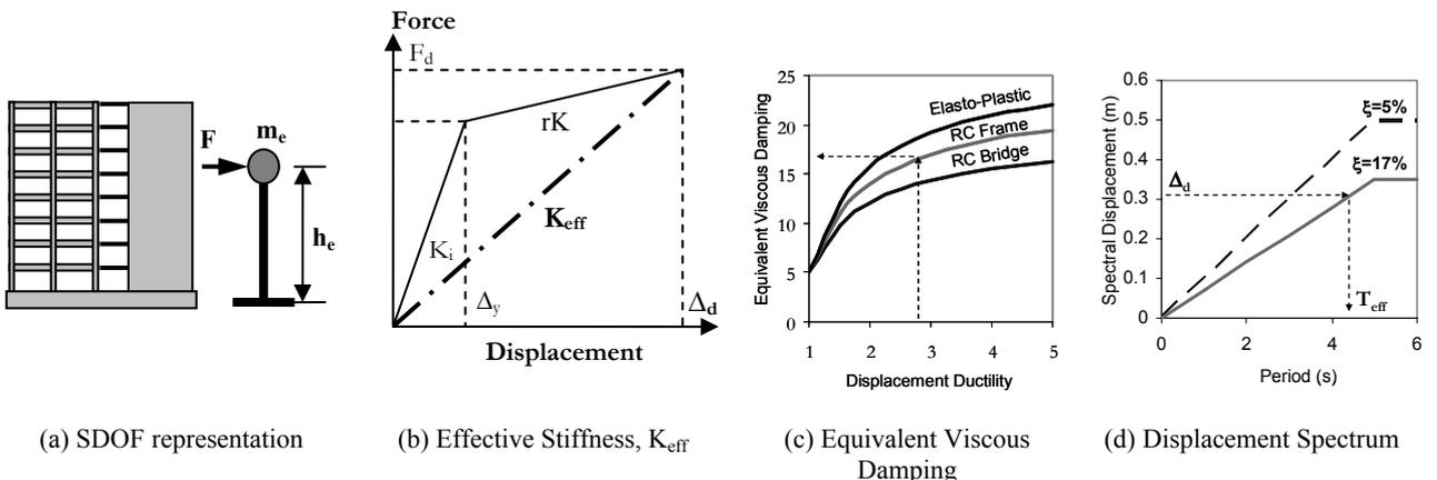
Figure 3: Fundamentals of Direct Displacement-Based Design (adapted from [3]).
