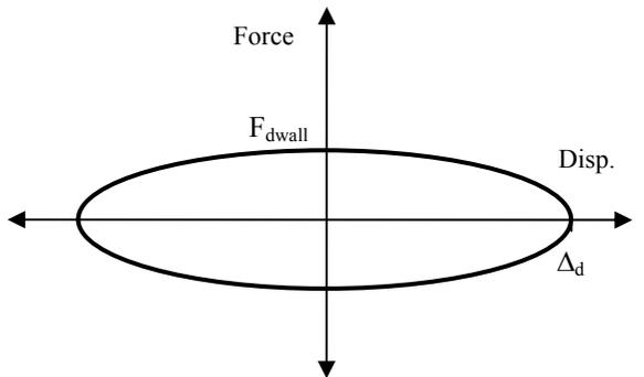
(b) Equivalent SDOF viscous damping
