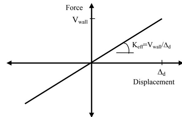
(c) Equivalent SDOF Effective Stiffness for RC walls
