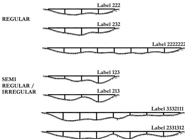
Figure 5: Bridge configurations.
