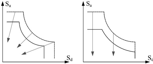
**Figure 1:** Spectral reduction methods: damping-based (left) and ductility-based (right).
