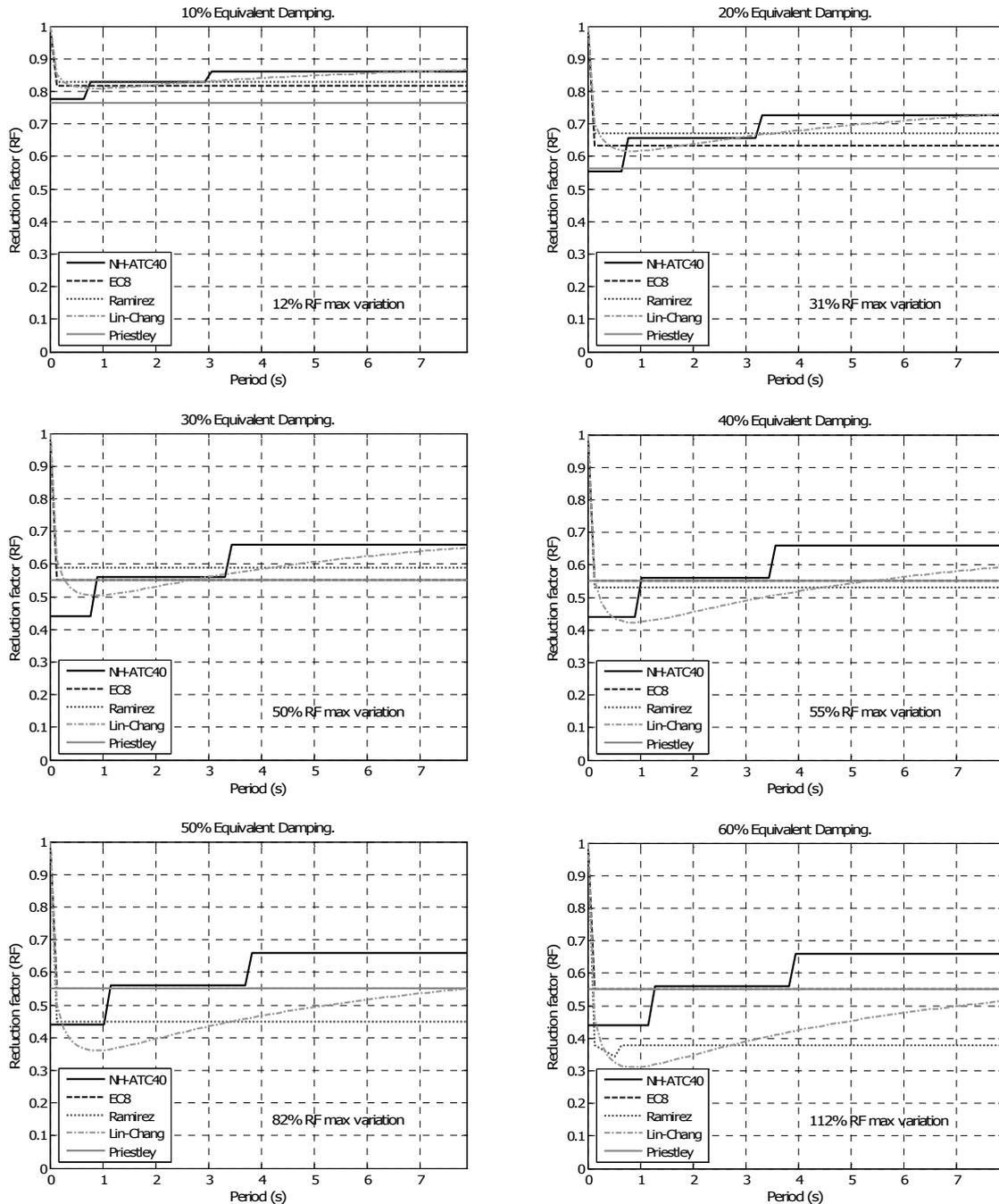
Figure 4: Reduction factor variation with period for different damping ratios.
