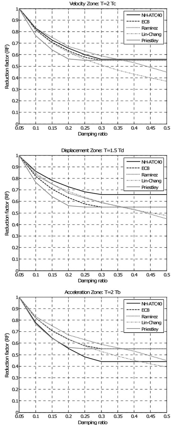
**Figure 3: Reduction factor variation with damping in the three spectral regions.**
