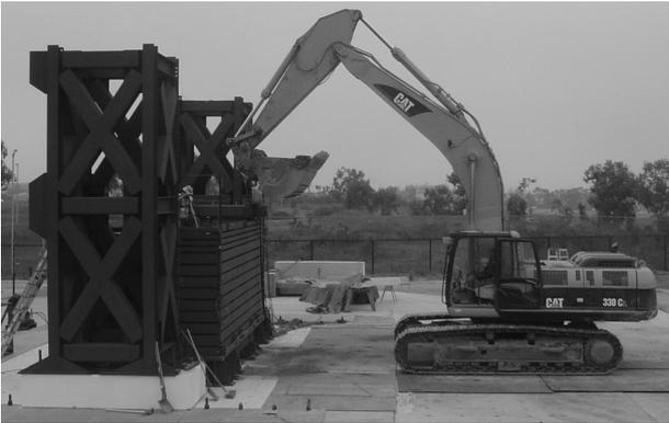
**Figure 2:** Soil model container on the NEES outdoor shake table at UCSD.
