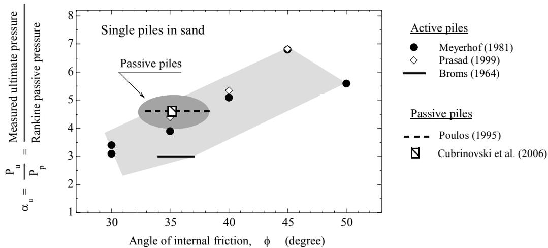
**Figure 8:** Ratio of ultimate pressure from the crust layer on a single pile and Rankine passive pressure obtained in experimental studies.
