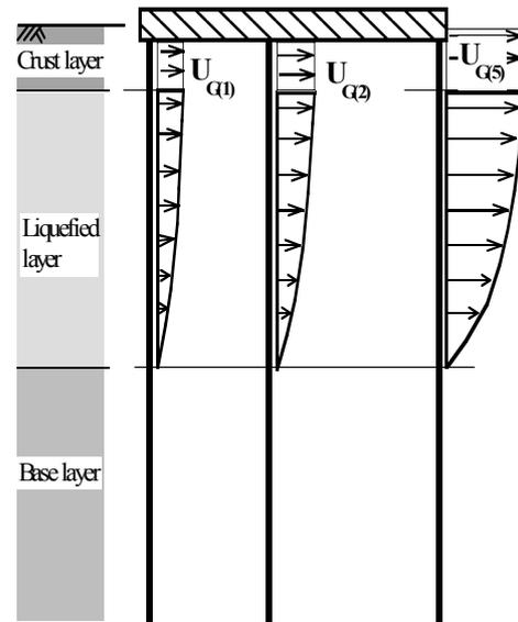
Figure 14: Non-uniform distribution of lateral spreading displacements acting on pile a group in the waterfront area.
