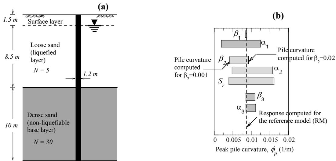
**Figure 13:** Effects of variation in soil parameters ( $\alpha_i$ ,  $\beta_i$  and  $S_r$ ) on the pile response: (a) Soil-pile model; (b) Tornado chart indicating the computed peak curvature of the pile for different values of key parameters.
