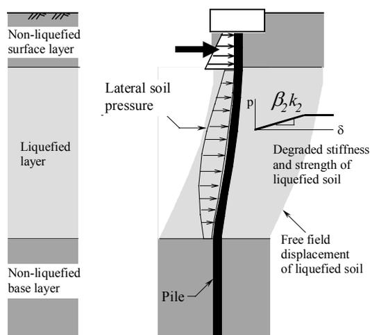
Figure 4: Three-layer deposit for piles in liquefied soils.
