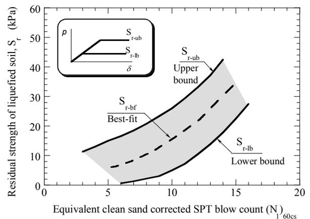
**Figure 12:** Residual strength ( $S_r$ ) of liquefied sandy soils back-calculated from case histories (after Seed and Harder, 1991).
