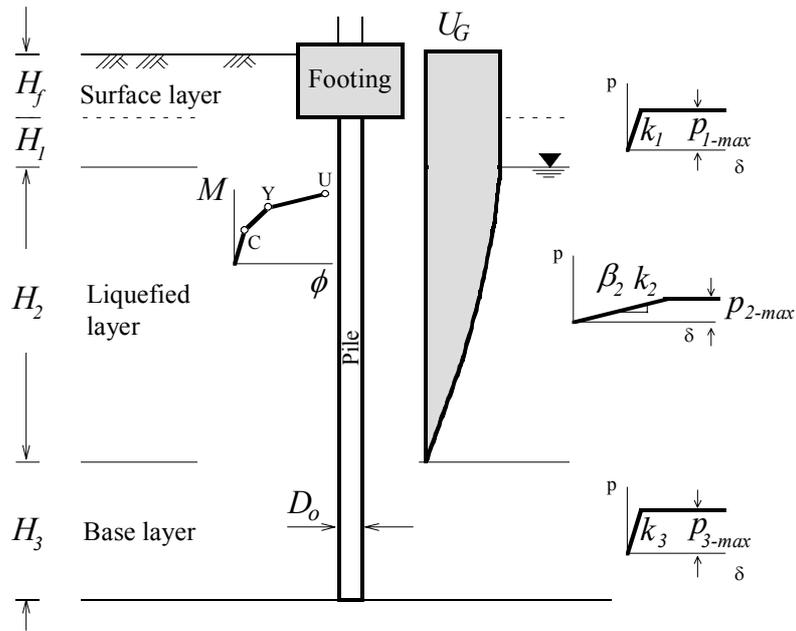
Figure 6: Characterization of load-deformation relationships and input parameters of the model.
