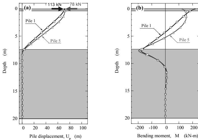
Figure 15: Illustration of cross-interaction effects on end piles subjected to different ground displacements (small ground displacement acting on Pile 1; large ground displacement acting on Pile 5): (a) Pile displacements, and (b) Bending moments.
