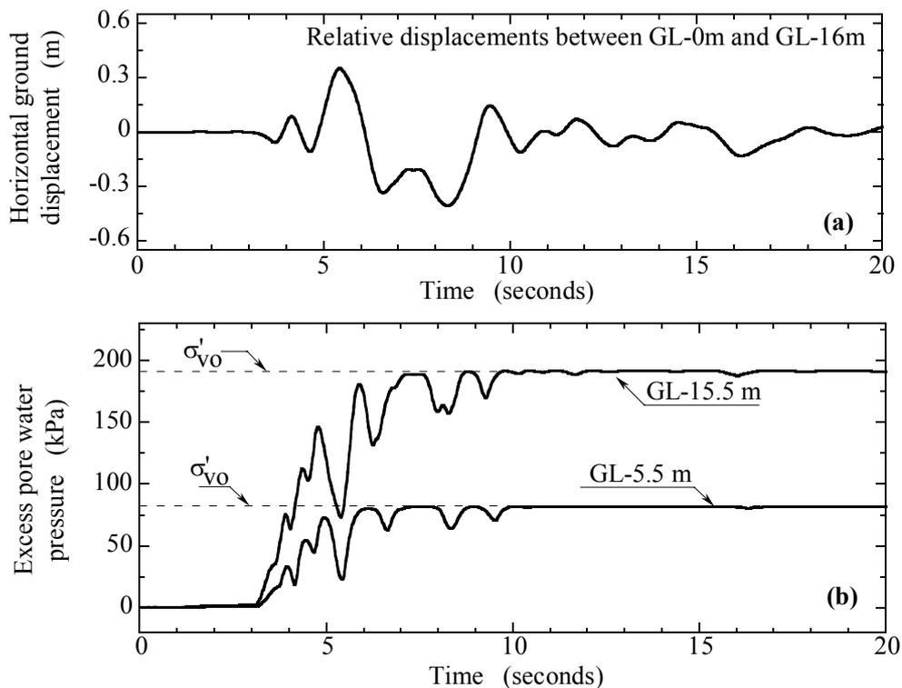
**Figure 1:** Ground response of liquefied deposit in the 1995 Kobe earthquake: (a) Cyclic ground displacement (relative displacement between ground surface and 16m depth); (b) Excess pore water pressure at 5.5m and 15.5m depth.
