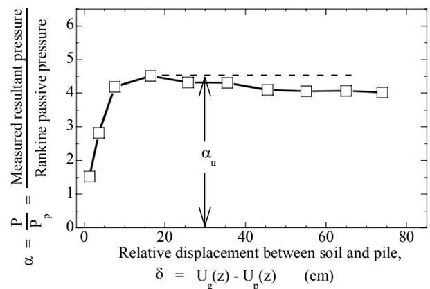
Figure 7: Ratio of lateral pressure from the crust layer on a single pile measured in a full-size test using large-scale shake table and Rankine passive pressure.
