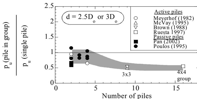
Figure 16: Reduction of lateral soil pressure due to pile-group effects.
