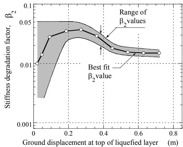
**Figure 11:** Degradation of stiffness in the liquefied layer observed in full-size test on piles.
