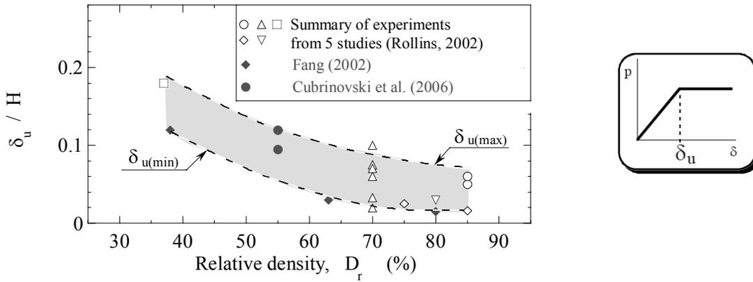
**Figure 10:** Relative displacement required to fully mobilize the passive pressure as a function of the relative density of sand: summary of data from experimental studies.
