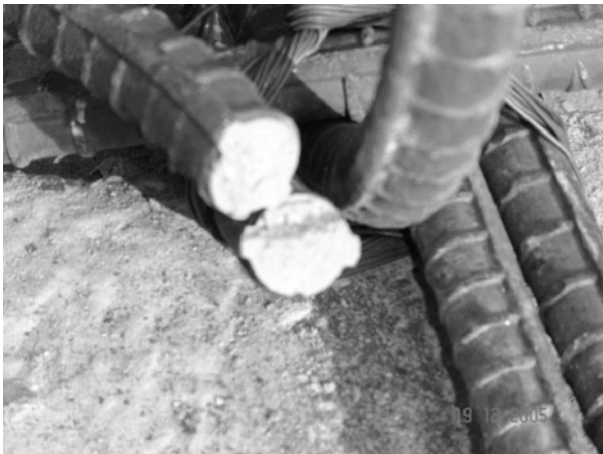
a). Snapping of reinforcement during bending.
