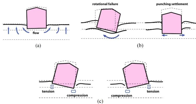
**Figure 1 - Liquefaction-induced mechanisms affecting settlement (Bray & Dashti, 2010)**
