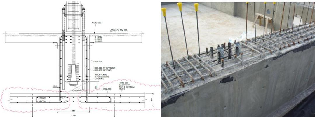
**Figure 4 - Typical detail of the adopted RC raft foundation**
