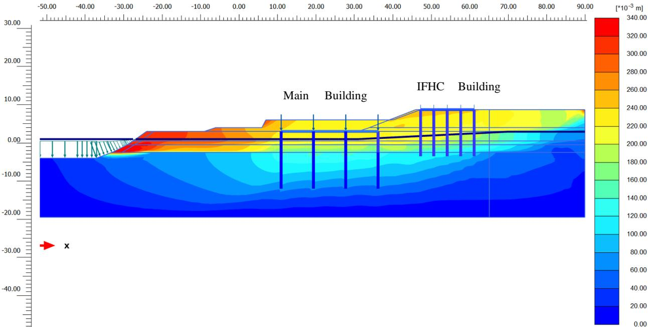
**Figure 6 - PLAXIS displacements for IL4 ULS event (displacements IFHC building platform are 235 mm to 245 mm)**
