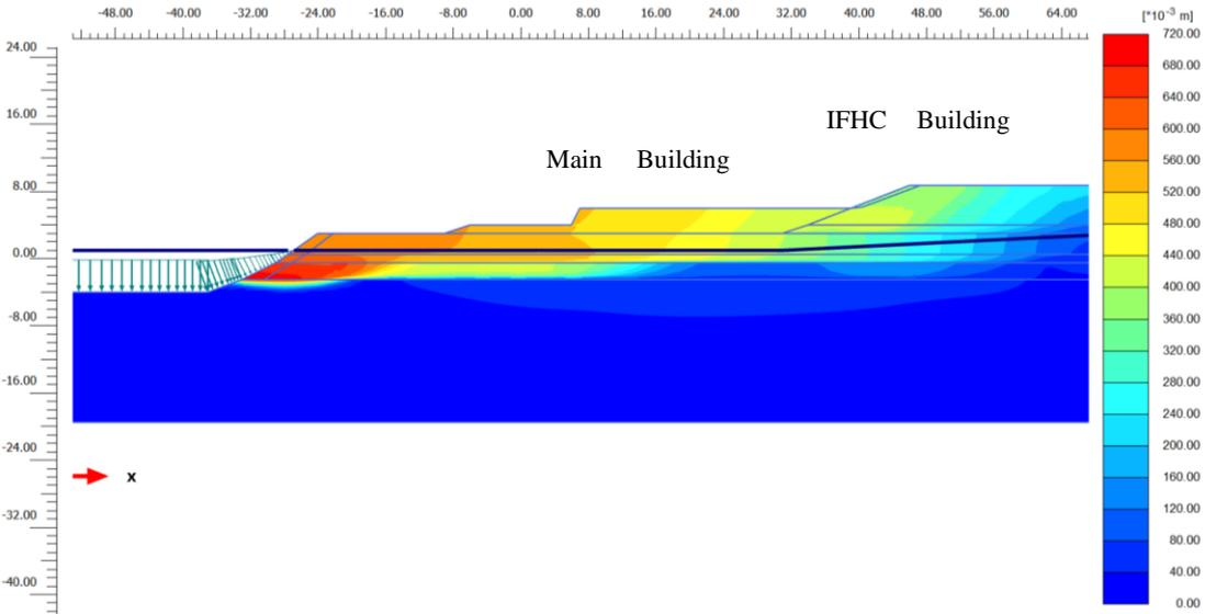
**Figure 5 - PLAXIS free-field displacement for IL3 ULS event (displacements are 400 mm to 510 mm at the Main Building platform)**
