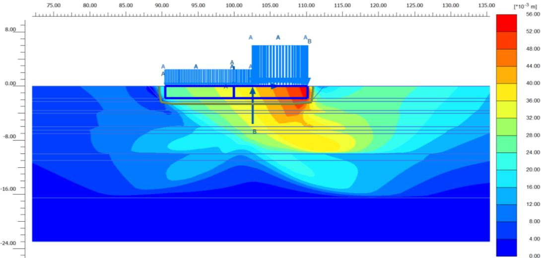
**Figure 3 - Vertical displacements from the seismic pushover analysis case with liquefaction**
