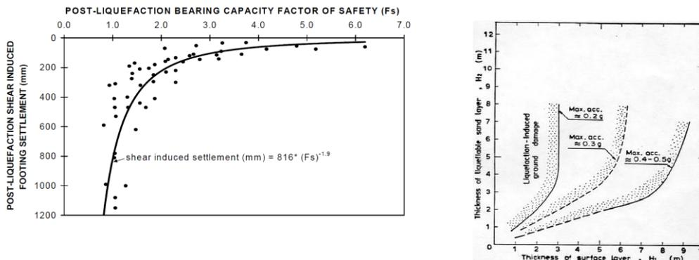
**Figure 2 - Correlation between post-liquefaction shear-induced settlement and post-liquefaction bearing capacity factor of safety, Naesgaard et al., 1998 (left); correlations for the assessment of liquefaction-induced damage, Ishihara, 1985 (right)**
