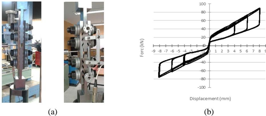
**Figure 3 - Experimental test of a double acting RSF joint a) Test setup; b) Hysteresis loops**
