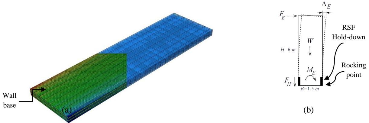
**Figure 4 - Numerical modelling of a CLT wall a) Assembly and stress distribution; b) Elastic deflection of the wall**
