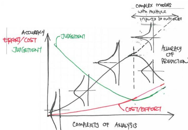
**Figure 4: Trade-off between accuracy, engineering judgement, cost and complexity of structural analysis**
