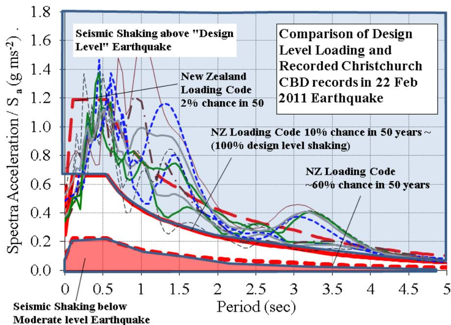
**Figure 3: Comparison of “Design Level” and Moderate Level Shaking (33%) with the recorded horizontal acceleration response spectra in Christchurch CBD from the 22 February 2011 earthquake.**
