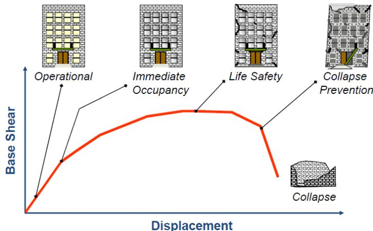
**Figure 2: Relationship of building response/damage to member response (Heintz et al, 2014)**
