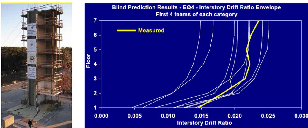
**Figure 5: UCSD, PCA & NEES blind prediction contest for a shaking table test of a full-scale reinforced concrete wall test building (image from Panagiotou and Restrepo, 2007)**
