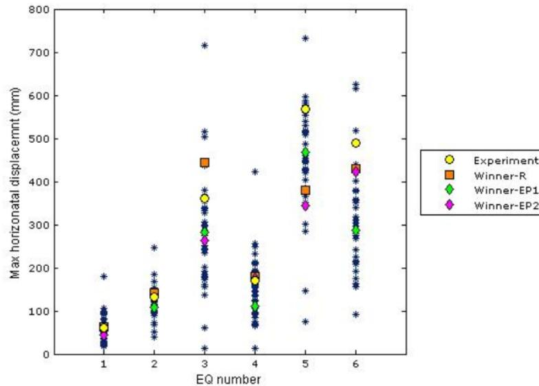
**Figure 6: PEER blind prediction experimental-prediction for shaking table test of a full-scale reinforced concrete column sub-assembly (PEER, 2010).**
