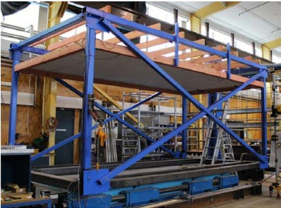
**Figure 4. Test frame on shake table.**
