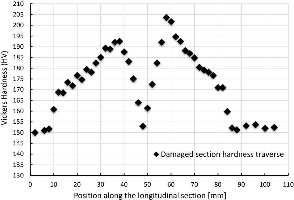
**Figure 9. Hardness longitudinal profile of the damaged re-bar obtained from building A.**
