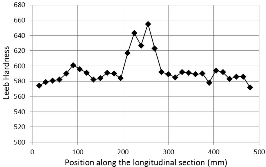
**Figure 4. Typical Leeb hardness profile of a damaged steel reinforcing bar from Building A.**
