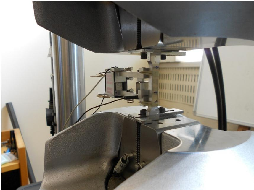
**Figure 10. Tensile testing of the damaged steel re-bar, the extensometer gauge length is measuring the strain in the damaged location.**
