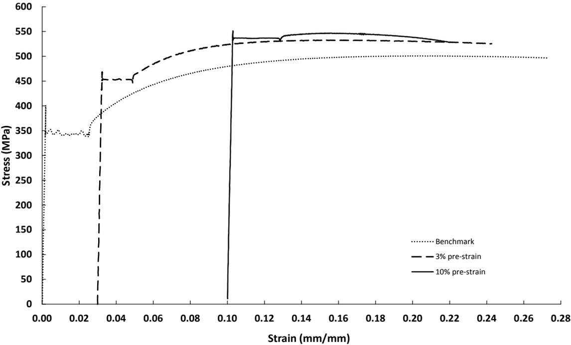
**Figure 6. Sample tensile stress-strain curves for baseline materials, 0.03 mm/mm pre-strain and age and 0.10 mm/mm pre-strain & age.**
