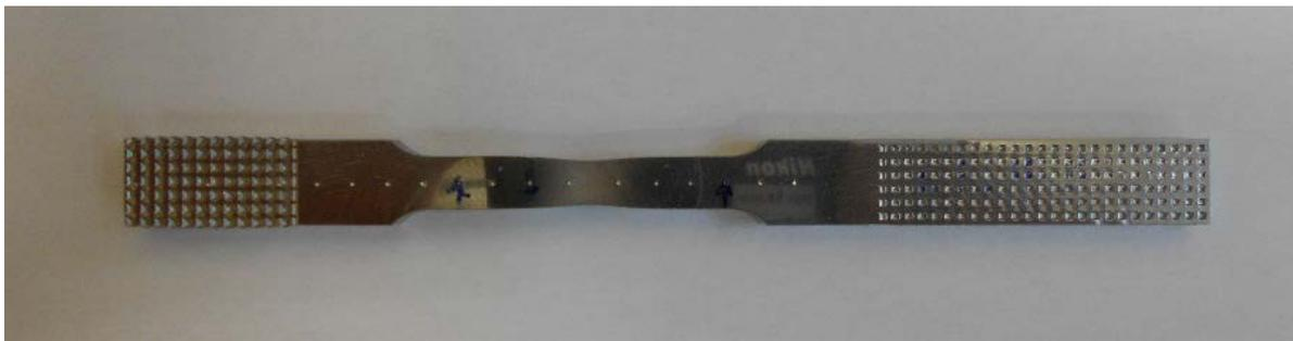
**Figure 11. The damaged samples after the final tensile test, the neck region corresponds to the area where the hardness was lower.**
