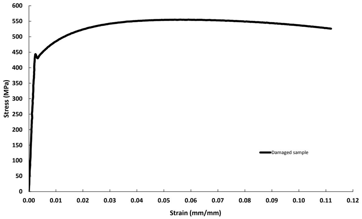
Figure 12. Stress-strain curve of the damaged steel re-bar.
