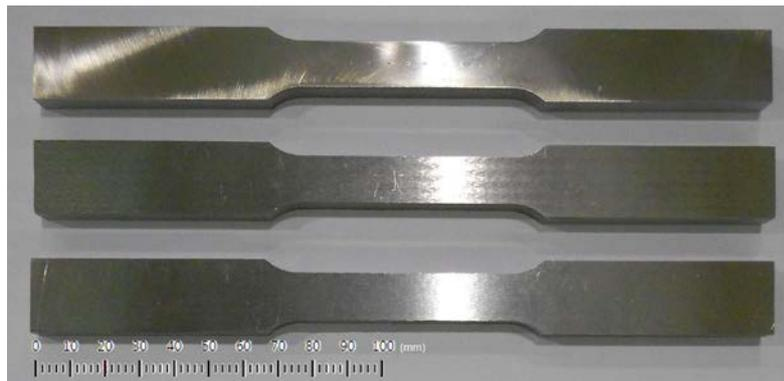
**Figure 5. “Dog-bone” steel specimen samples.**
