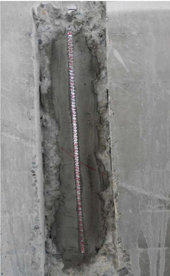
**Figure 2. Steel reinforcing bar exposed for and prepared for Leeb hardness testing.**
