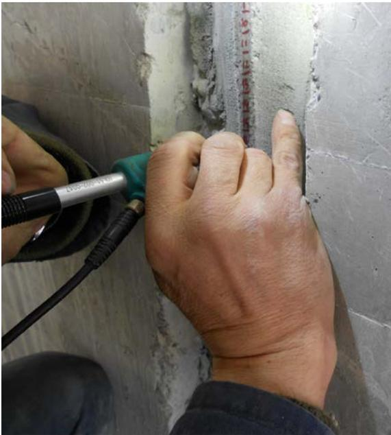
**Figure 3. Leeb hardness testing.**
