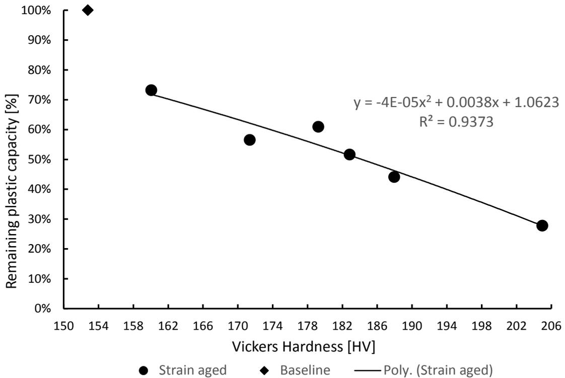
Figure 8. Remaining ductility versus Vickers hardness calibration curve for the un-damaged steel re-bar obtained from building A.
