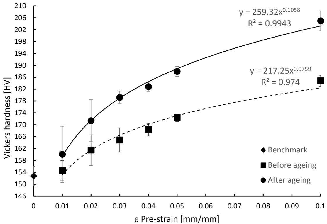
Figure 7. Hardness versus pre-strain calibration curve for the un-damaged steel re-bar obtained from building A.
