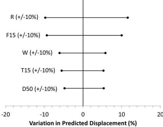
Figure 7. Sensitivity of Youd model relative to 10% change in input parameters
