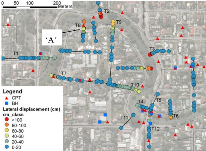
Figure 1. Lateral spreading field measurements in the Avon Loop following the 2011 Christchurch earthquake and location of site ‘A’ used in the subsequently discussed sensitivity analysis
