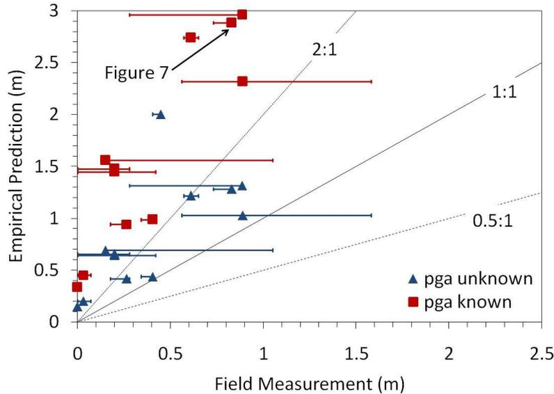
Figure 5. Comparison of field measurements of lateral displacements in the Avon Loop area with empirical predictions from the Youd et al. (2002) model
