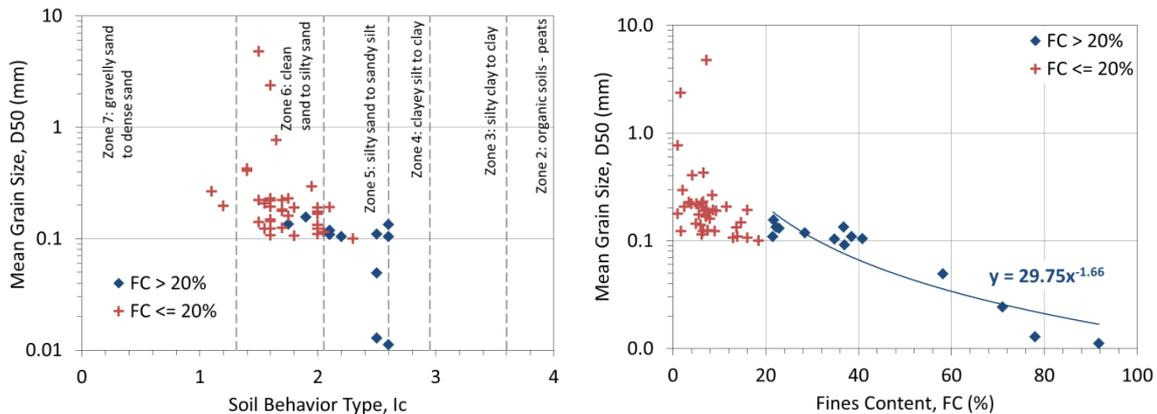
Figure 4. Relationship for Christchurch soils between mean grain size,  $D_{50}$ , and (a) Soil behaviour type,  $I_c$  and (b) Fines content,  $FC$
