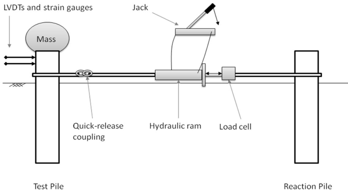
Figure 1. Schematic of snap-back test procedure
