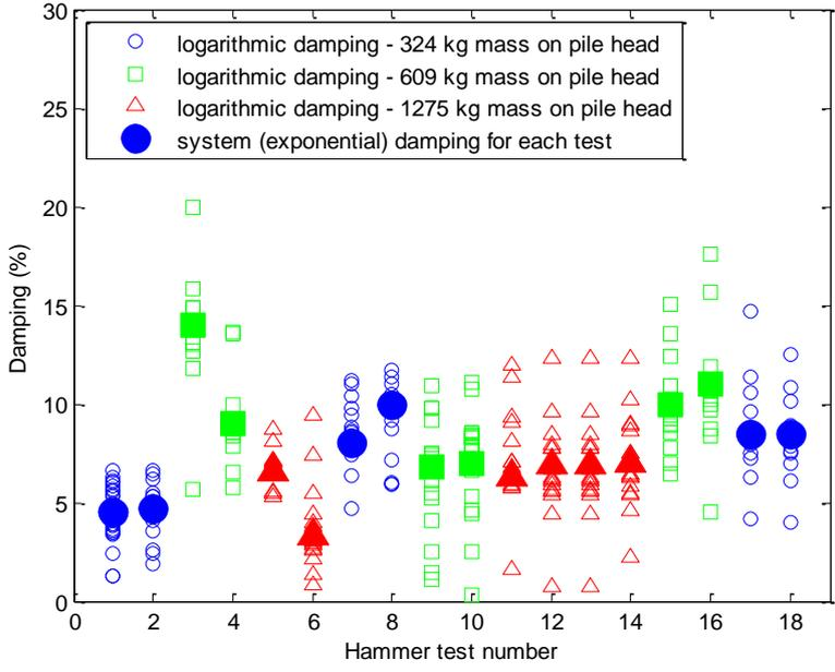
**Figure 3. Damping ratios computed from hammer tests using the logarithmic decrement method and exponential system damping envelopes.**
