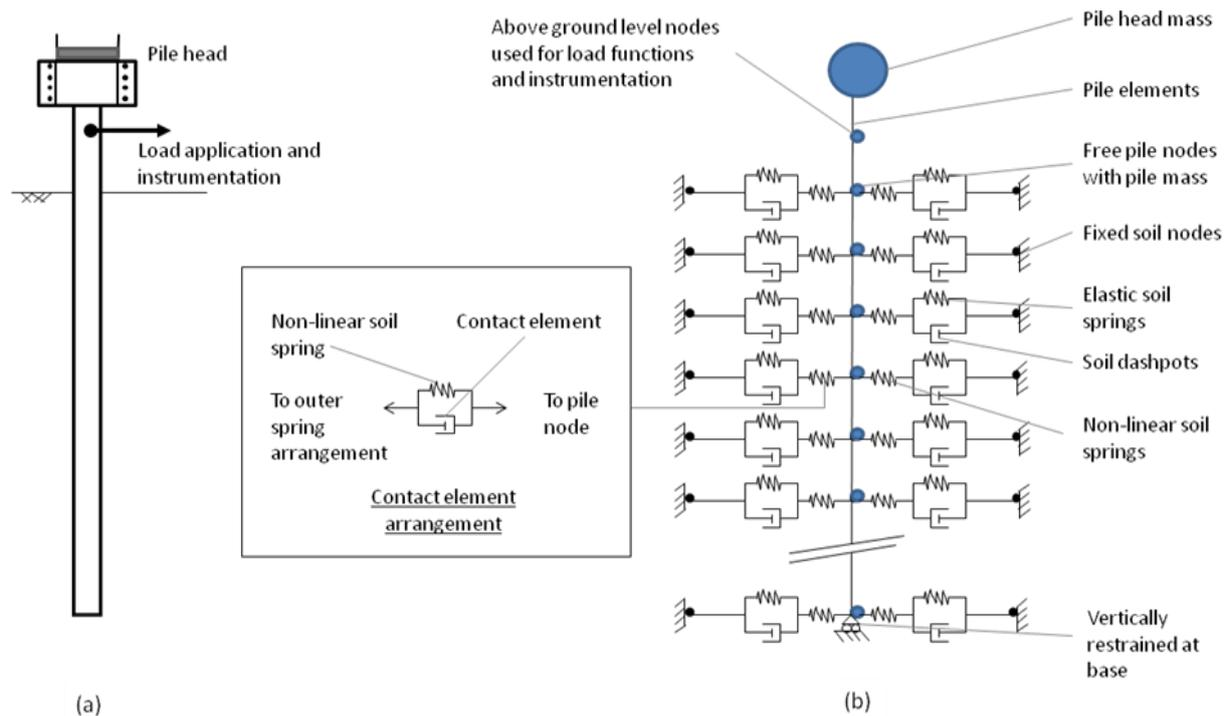
Figure 5. (a) Field testing set-up; (b) Numerical Winkler Spring model representation.
