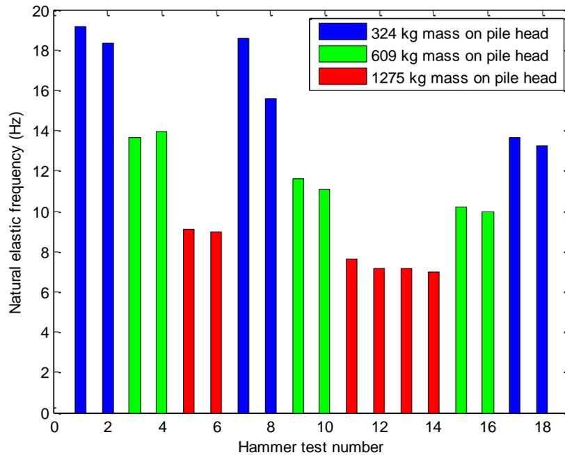
**Figure 2. Natural elastic frequencies of the test pile determined from FFT hammer response**
