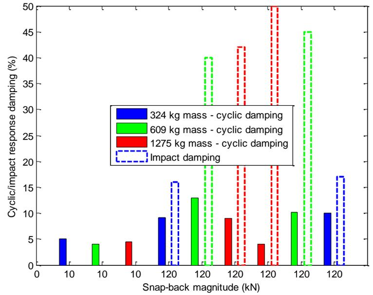
**Figure 4. Exponential system damping for all snap-back tests, illustrating snap-back order.**
