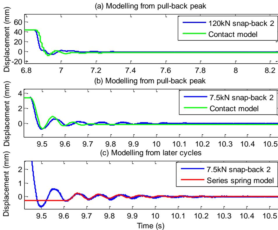
Figure 6. Ruaumoko contact and series spring model comparison on Pile 2 with (a) 120 kN snap-back from start of test; (b) 7.5 kN snap-back from start of test; (c) 7.5 kN snap-back from third peak.
