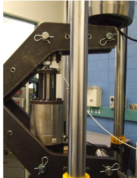
b) Lever-system to increase force capacity
