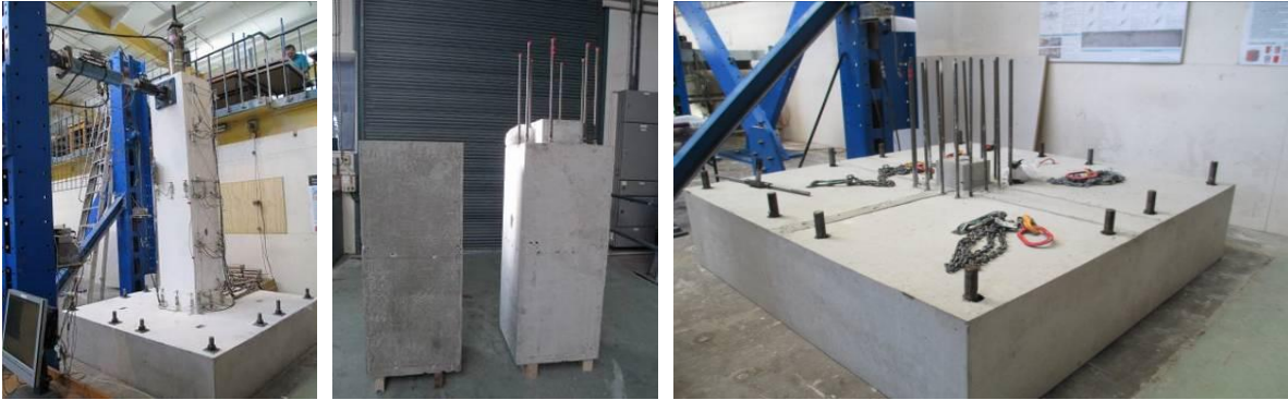
Figure 4 Assembled specimen SQ1 (left); segmental columns (middle); spread footing (right)
