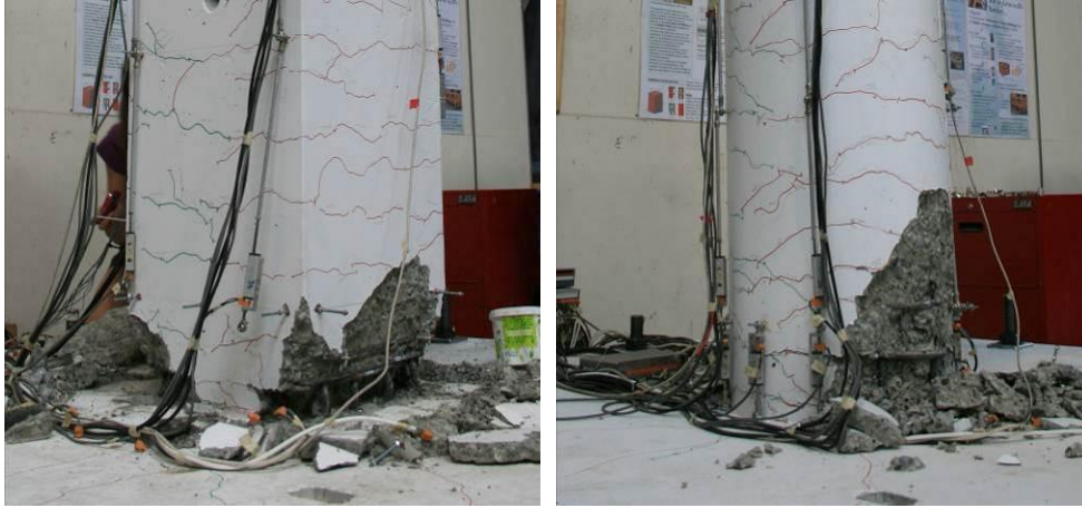
Figure 9 Plastic hinging of the base; SQ1 at 5% drift (left); CR1 at 6% drift (right)
