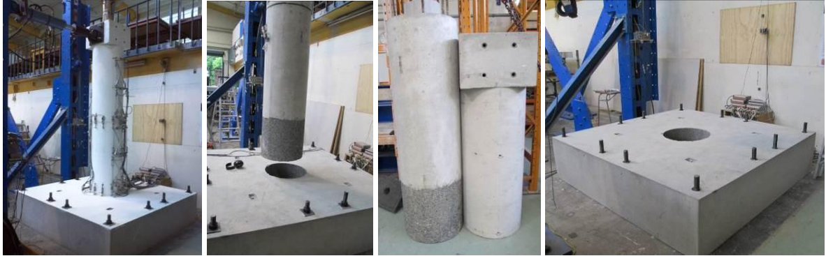
Figure 5 Assembled specimen CR1 (left); segmental columns (middle); spread footing (right)
