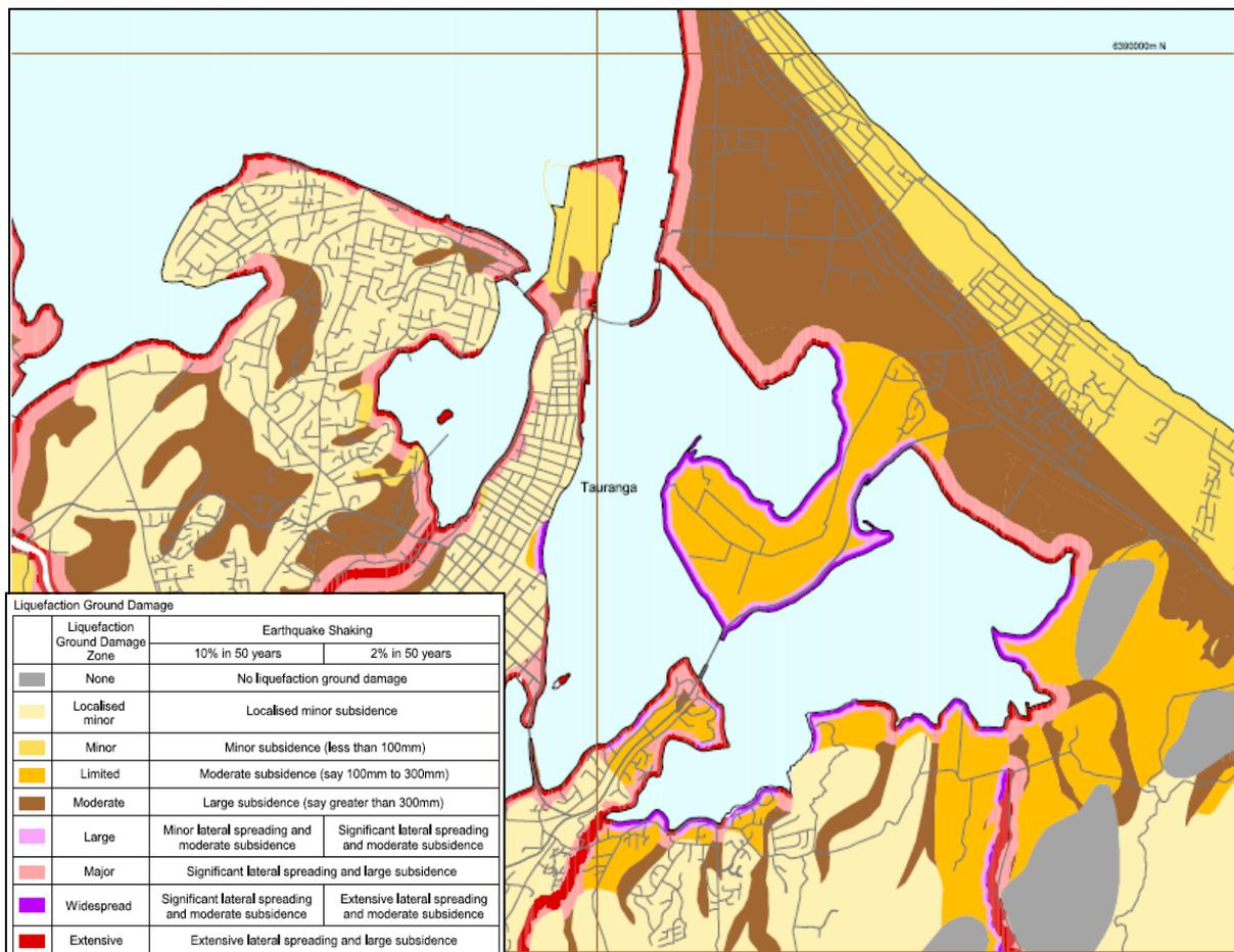
Figure 4. Liquefaction ground damage map extract for Western Bay of Plenty
