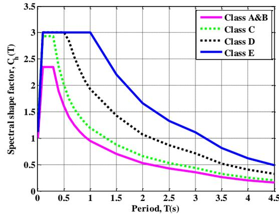
Figure 1: Spectral shape factor in NZS1170.5
