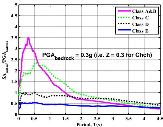
Figure 3: Spectral shape curves for different soil classes
