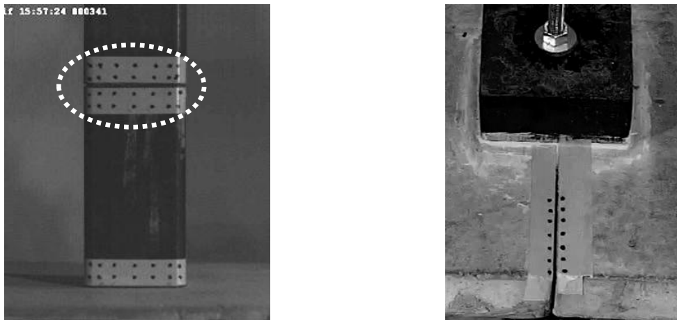
Figure 5: Zoom in of the cameras view: pier view with in evidence the rocking section analysed on the left and deck view on the right
