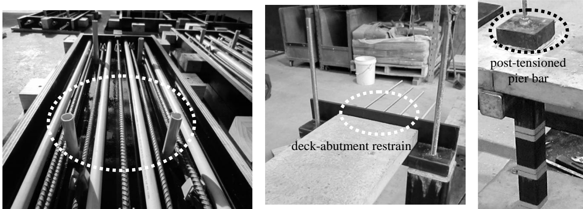
Figure 3: – Left: Close up of deck mould with longitudinal reinforcement horizontal and vertical ducts; Centre and Right: close up of the deck and pier assembly.
