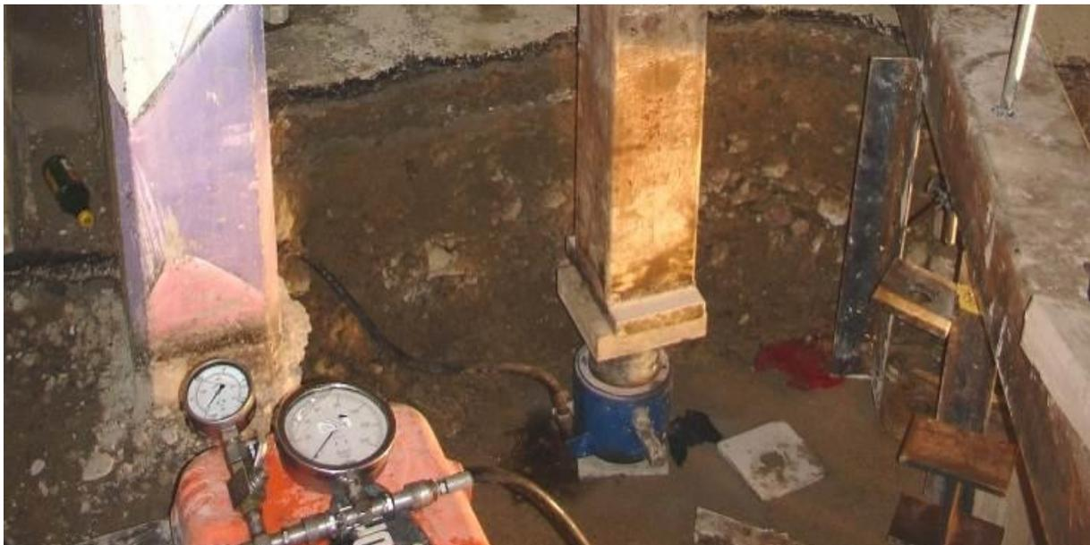
The tension failure of one of the test piles due to a structural defect threw into question the robustness of a primary structure reliant on piles only. A series of “what if” scenarios were investigated, considering a defect in one, two or three piles in a building. The total loss in overturning capacity was only 10-25%, and as such, the risk was considered acceptable without further investigation.
