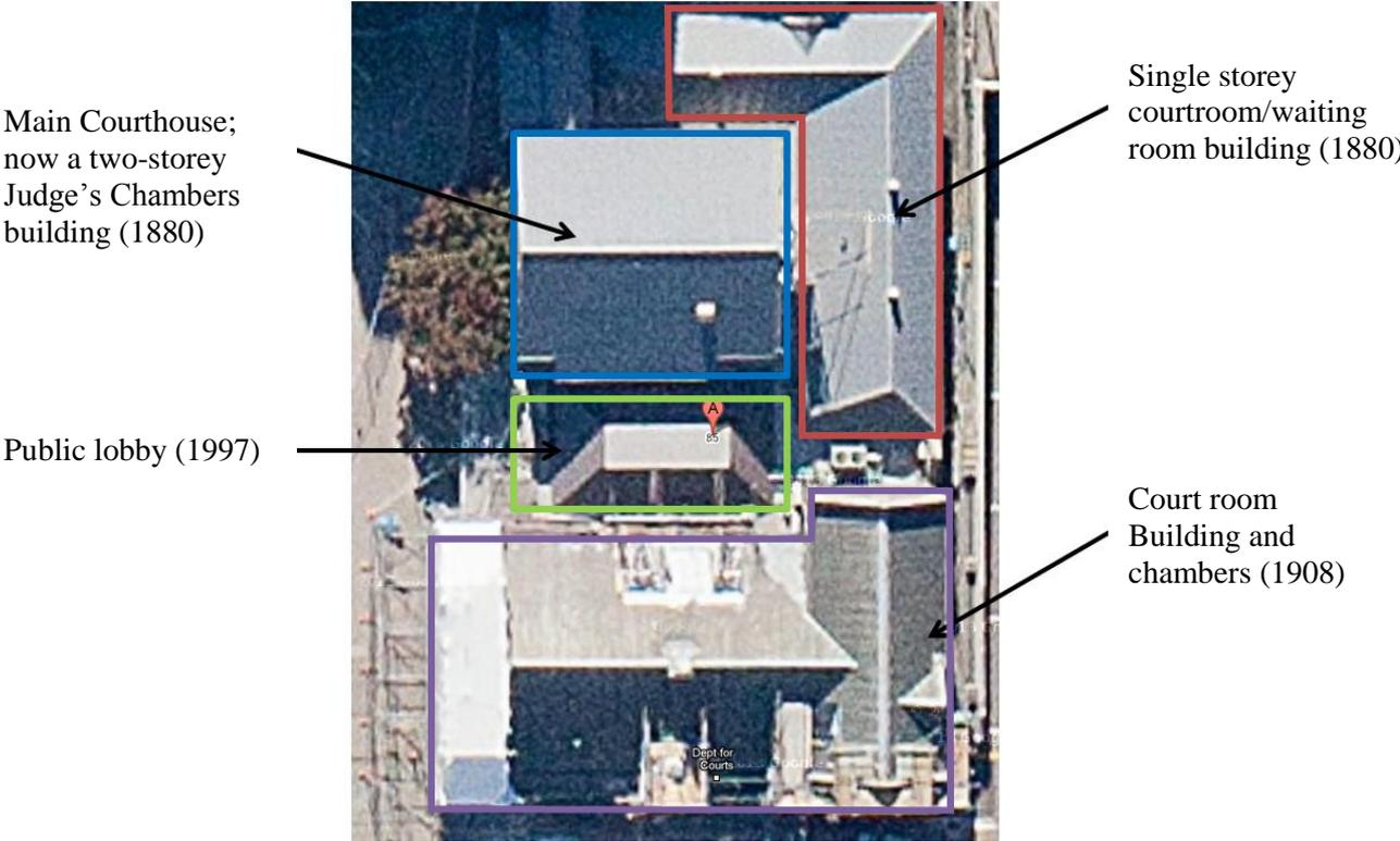
Figure 1.1: Aerial image showing the staged construction of the building (image courtesy Google Earth)
