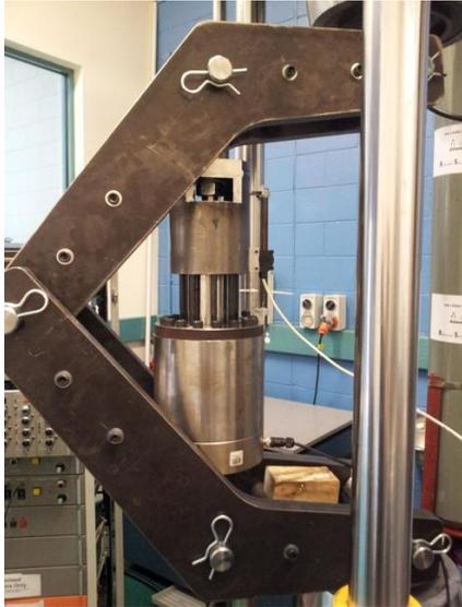
**Figure 21:** High Speed Testing of Devices at Quest Laboratory, showing lead damper and lever system
