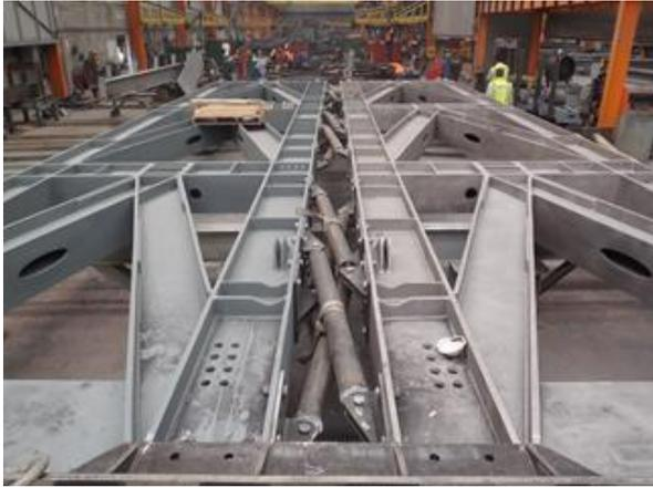
**Figure 6:** Pair of steel braced frames assembled in the workshop with dampers
