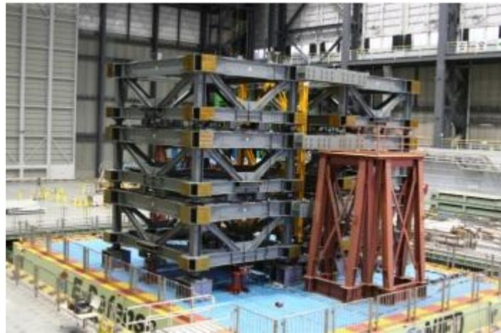
**Figure 3:** Shake Table Testing of Steel Self-Centering Braced Frames at the E-Defence Shake Table in Japan (Deierlein et al. 2010)
