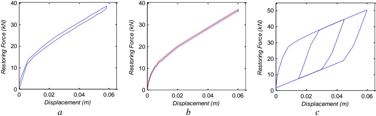
Figure 2 Force-displacement response - a) experimental SRW; b) numerical SRW approximation; and c) numerical SRW with mild steel hysteretic dampers
