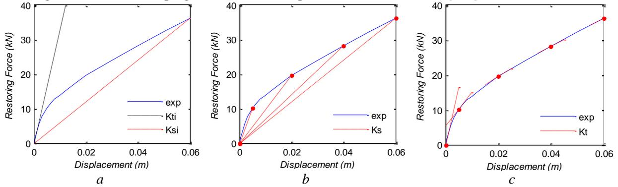
Figure 6 The four stiffness schemes – a) initial tangent and secant, b) updated secant, and c) updated tangent
