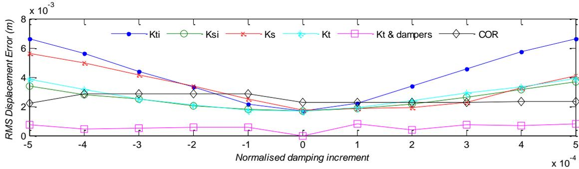
Figure 11 Root mean square of displacement error with respect to variation in damping ratio away from optimal value
