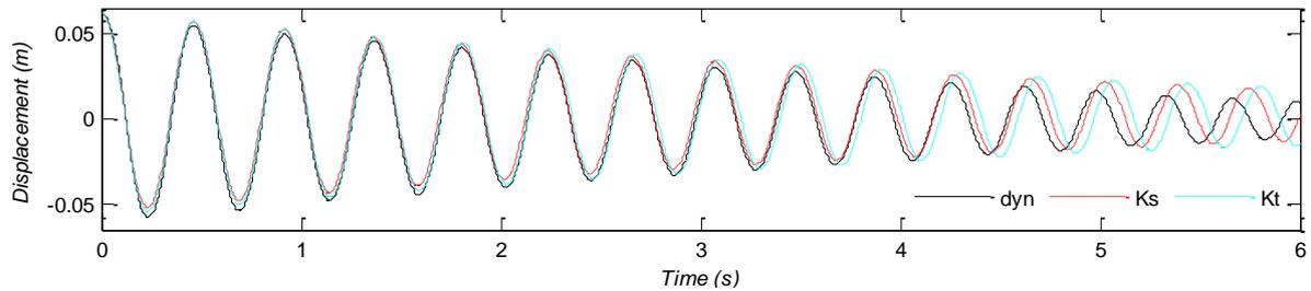
Figure 13 PSD snapback displacement time histories with revised damping coefficients
