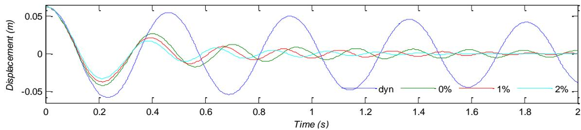
Figure 15 Snapback displacement time history for SRW wall with mild steel dampers and three tangent stiffness proportional EVD analyses compared to dynamic SRW response
