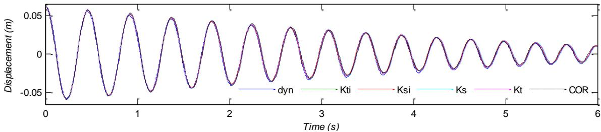
Figure 9 Best fit numerical displacement time histories for the five damping schemes compared to the actual dynamic response
