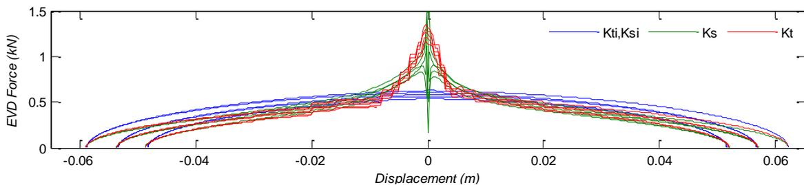
Figure 10 EVD force as a function of displacement for the four optimised damping schemes over the first three oscillations (others omitted for clarity)
