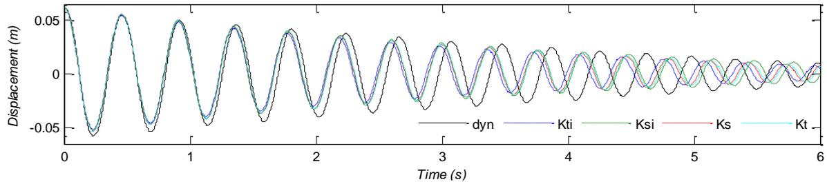
Figure 12 PSD snapback displacement time histories with numerically optimised damping coefficients
