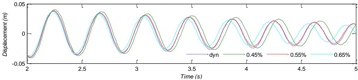
Figure 8 Numerical displacement time histories for analyses adopting updating tangent stiffness proportional EVD and friction compared to the actual dynamic response
