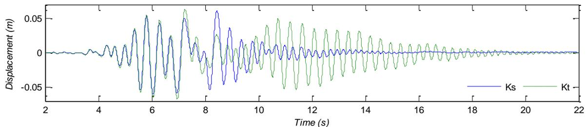
Figure 14 PSD response to the REHS earthquake record for the optimised updating EVD schemes
