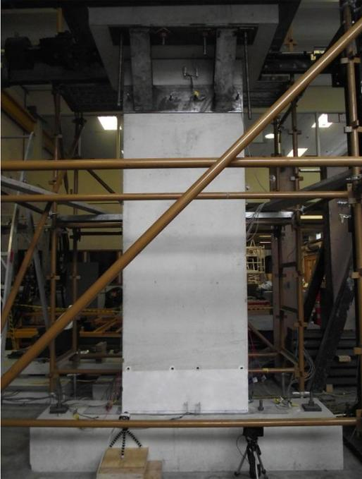
Figure 1 The SRW setup for testing
