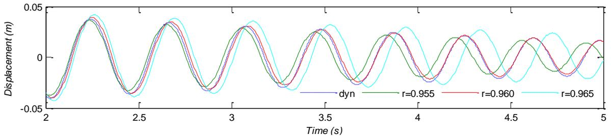
Figure 5 Numerical displacement time histories implementing damping via constant Coulomb friction and COR
