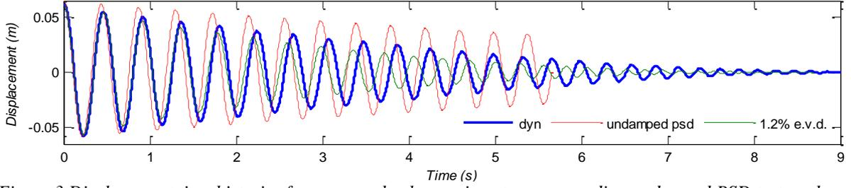
Figure 3 Displacement time histories from a snap back experiment, corresponding undamped PSD test, and corresponding PSD test with 1.2 % initial secant stiffness proportional EVD
