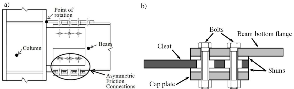
Figure 1. (a) Sliding Hinge Joint (MacRae et al. (2010)) and (b) Asymmetric Friction Connection
