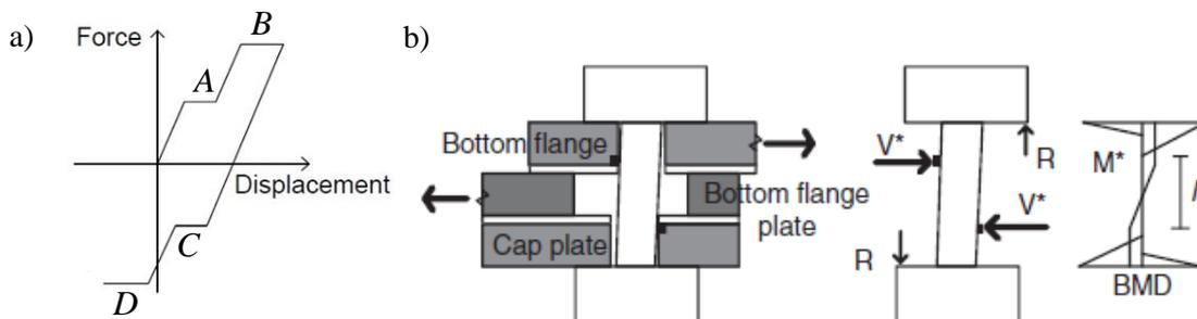
**Figure 2. Idealised (a) force-displacement curve (Khoo et al. (2012a)) and (b) bolt behaviour during sliding (Khoo et al. (2012a))**
