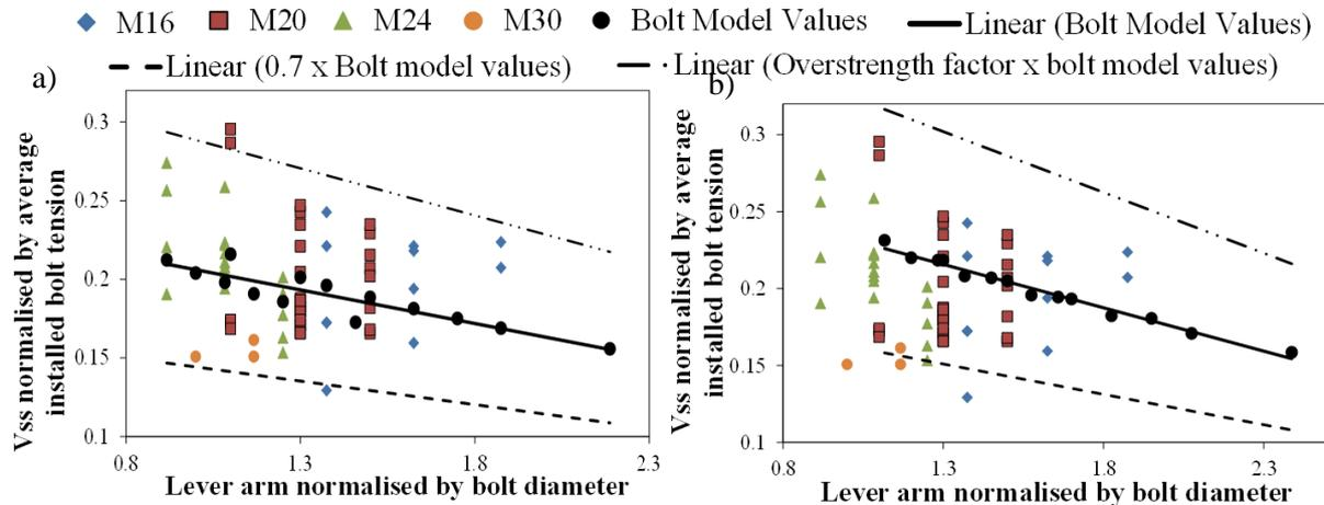
Figure 9. (a) Experimental  $V_{ss}$  with revised bolt model predictions and (b) experimental  $V_{ss}$  with MacRae et al. (2010) bolt model predictions
