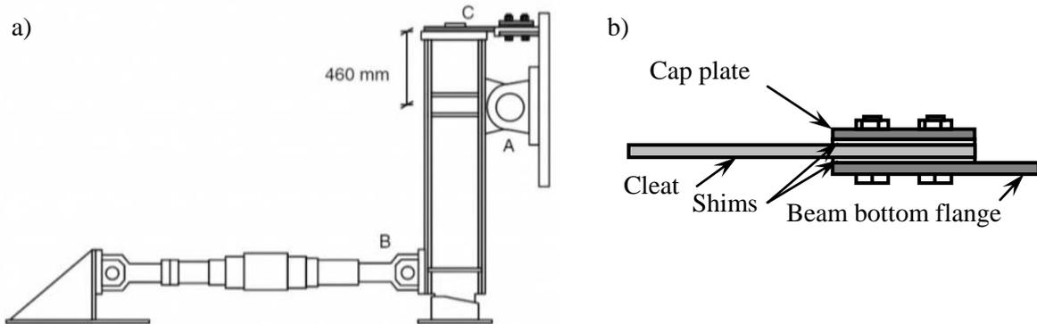
Figure 3. (a) Test setup (Khoo et al. (2012a)) and (b) AFC configuration during testing
