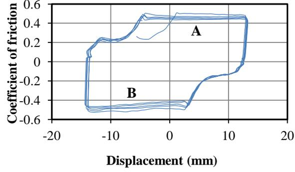
Figure 7. Coefficient of friction for M20 bolt and 20mm cleat
