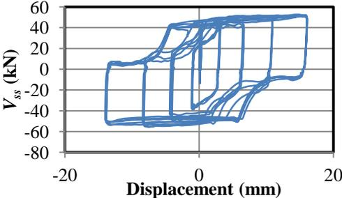
**Figure 5. Hysteresis curve for M16 bolts and 16 mm cleat**
