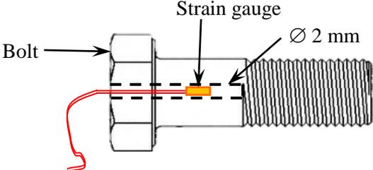
**Figure 4. Strain gauge in bolt**
